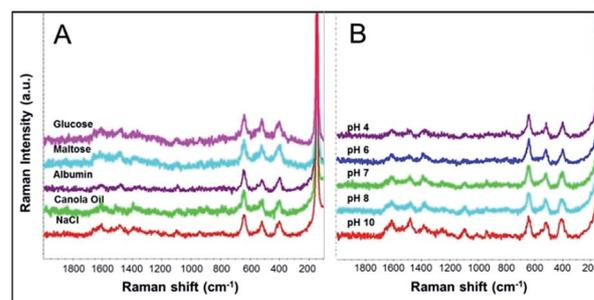
Fig. 6 Effects of complex matrices on MYC-assisted and SERS detection for  $\text{TiO}_2$  NPs analysis, including various interferences (A) and pH conditions (B). The concentration of  $\text{TiO}_2$  NPs for all cases is  $200 \text{ mg L}^{-1}$ .
