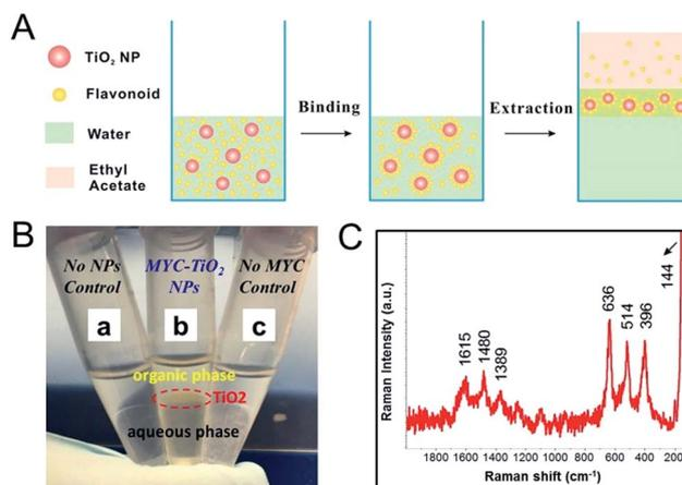
Fig. 4 (A) Schematic illustration of flavonoid-assisted microextraction method for TiO<sub>2</sub> NPs from water. (B) Photographs of flavonoid-based phase separation. Selected flavonoid is MYC. (C) SERS spectra of MYC-adsorbed TiO<sub>2</sub> NPs from the interlayer. NP = nanoparticle.
