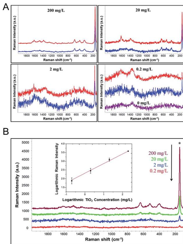
Fig. 5 (A) SERS spectra of different concentrations of  $\text{TiO}_2$  NPs with (blue curves) and without extraction (red curves). No  $\text{TiO}_2$  NPs control ( $0 \text{ mg L}^{-1}$ ) is also shown (purple curve). (B) SERS spectra of extracted  $\text{TiO}_2$  NPs using MYC-assisted extraction method. Inset: linear fitting curve for quantification of extracted  $\text{TiO}_2$  NPs based on  $144 \text{ cm}^{-1}$  Raman peak.
