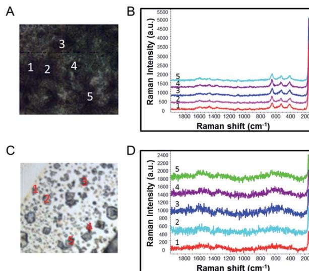
Fig. 3 (A) Photograph of TiO<sub>2</sub> NPs sample (200 mg L<sup>-1</sup>) on gold slide. 20× microscope objective was used. (B) SERS spectra of selected positions in (A). (C) Photograph of TiO<sub>2</sub> NPs sample (2 mg L<sup>-1</sup>) on gold slide. (D) SERS spectra of selected positions in (C).
