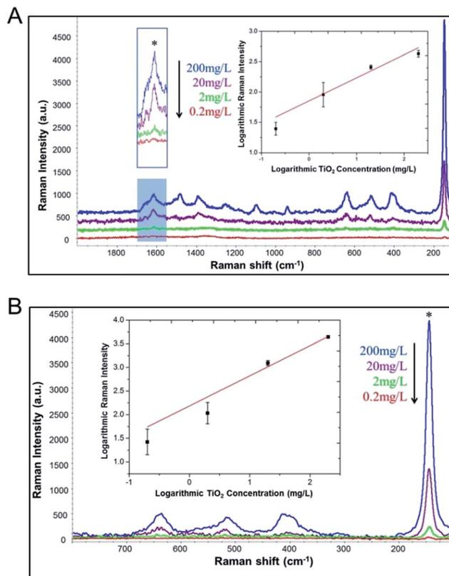
Fig. 2 (A) SERS spectra of MYC-adsorbed TiO<sub>2</sub> NPs with various concentration. Inset: linear fitting curve for MYC-adsorbed TiO<sub>2</sub> NPs detection based on 1615 cm<sup>-1</sup> peak of MYC indicated with asterisk. (B) Raman characteristic peaks of TiO<sub>2</sub> NPs in the range from 100–800 cm<sup>-1</sup>. Inset: linear fitting curve for quantification of TiO<sub>2</sub> NPs based on 144 cm<sup>-1</sup> Raman peak.
