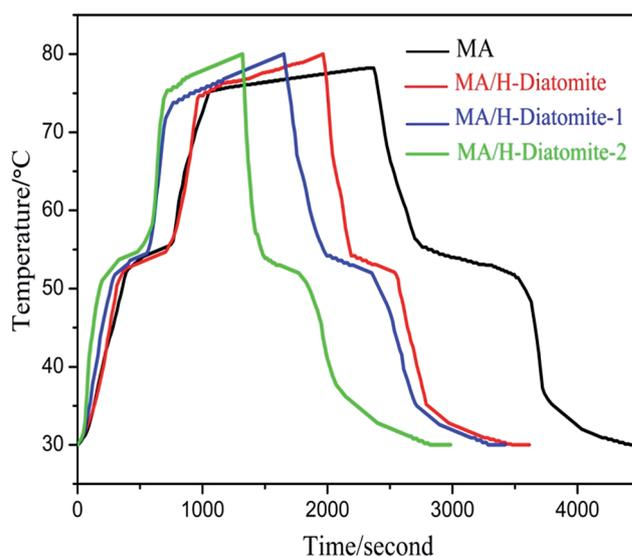
Fig. 6 Thermal storage and release curves of MA, MA/H-diatomite, MA/H-diatomite-1, and MA/H-diatomite-2.
