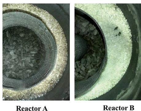
Fig. 3 Evidence of secondary cracking through color change on particles in the vicinity of the reactor wall for reactors A and B.
