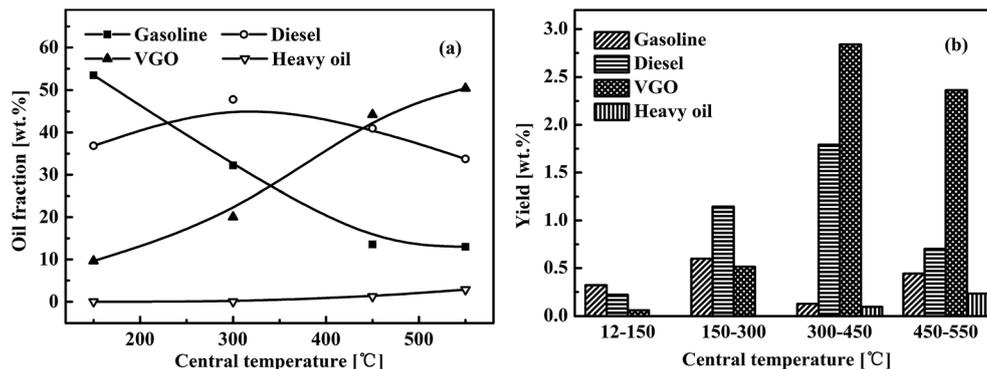
Fig. 5 Variations in (a) oil fraction and (b) yield with changing central temperature in the reactor with internals.
