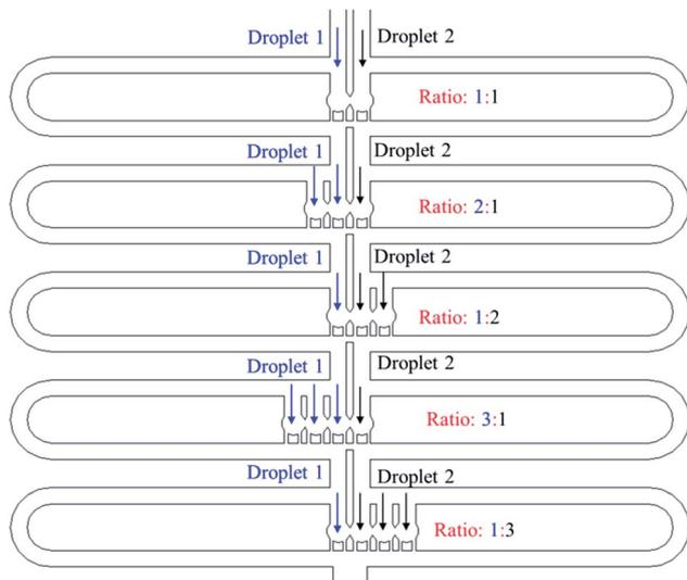
**Fig. 8** Sketch of the trapping well design for trapping multiple droplets with a concentration gradient of reagents. The number of trapped droplets ratio in a trapping well varies from 1 : 3 to 3 : 1, which creates 5 different reagent concentrations.
