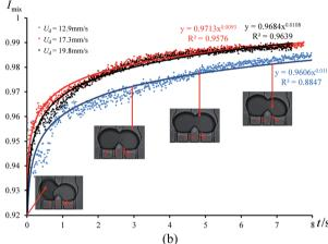
Fig. 6 (a) Grayscale value measurement area, where the boundary was excluded. The scale bar is 100  $\mu$ m. (b) Mixing index vs. time under different droplet average velocities.
