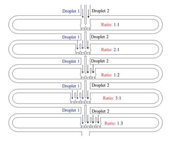
Fig. 8 Sketch of the trapping well design for trapping multiple droplets with a concentration gradient of reagents. The number of trapped droplets ratio in a trapping well varies from 1:3 to 3:1, which creates 5 different reagent concentrations.
