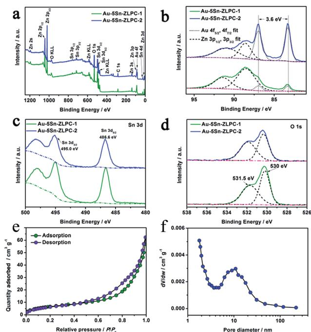
Fig. 6 (a) XPS spectra and (b–d) high resolution XPS spectra of Au-5Sn-ZLPCs at binding energies corresponding to Au 4f, Sn 3d and O 1s, respectively. (e)  $N_2$  adsorption-desorption isotherm and (f) the BJH pore size distribution calculated from adsorption branches of Au-5Sn-ZLPC-2.
