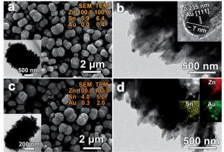
SEM, TEM images and EDS results of 5.0 at% Sn-ZLPC decorated by different amounts of Au: (a, b) Au-5Sn-ZLPC-1 (insets are corresponding TEM and HRTEM images), (c, d) Au-5Sn-ZLPC-2 (insets are corresponding TEM and EDS mapping images).
