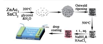
Fig. 4 Schematic illustration of the preparation of Au–5Sn–ZLPCs gas sensors.
