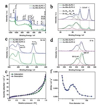
Fig. 6 (a) XPS spectra and (b-d) high resolution XPS spectra of Au-5Sn-ZLPCs at binding energies corresponding to Au 4f, Sn 3d and O 1s, respectively. (e) N<sub>2</sub> adsorption-desorption isotherm and (f) the BJH pore size distribution calculated from adsorption branches of Au-5Sn-ZLPC-2.
