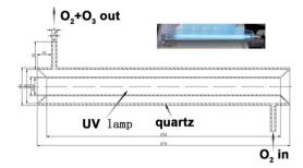
Fig. 1 Schematic diagram (the cross-sectional view) of the experimental set-up used to produce ozone gas (the inset is a digital photograph of the experimental set-up).
