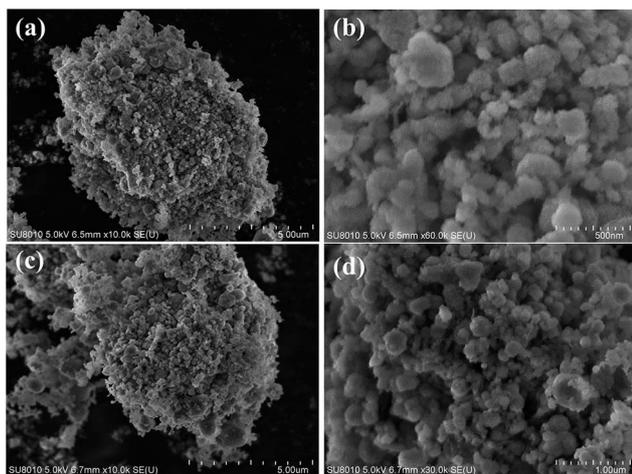
Fig. 14 SEM images of (a and b) 0.6Pt/meso-Co<sub>3</sub>O<sub>4</sub> catalyst and (c and d) the used 0.6Pt/meso-Co<sub>3</sub>O<sub>4</sub>.
