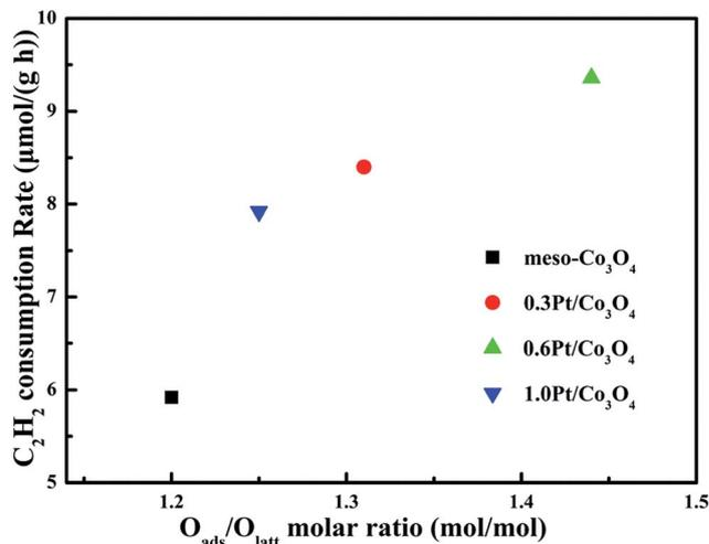
Fig. 12 Acetylene consumption rates at 60 °C as a function of O<sub>ads</sub>/O<sub>latt</sub> molar ratio of meso-Co<sub>3</sub>O<sub>4</sub>, 0.3Pt/meso-Co<sub>3</sub>O<sub>4</sub>, 0.6Pt/meso-Co<sub>3</sub>O<sub>4</sub> and 1.0Pt/meso-Co<sub>3</sub>O<sub>4</sub>. Reaction gas composition: [C<sub>2</sub>H<sub>2</sub>] = 50 ppm, [O<sub>2</sub>] = 13 vol%, N<sub>2</sub> balance and GHSV = 30 000 h<sup>-1</sup>.
