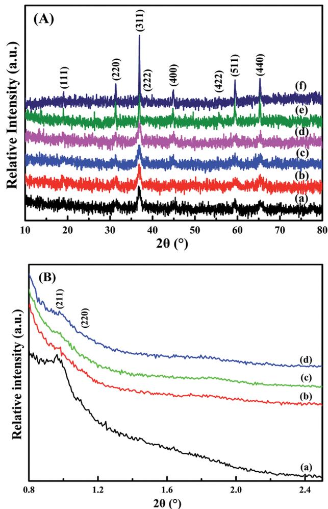
Fig. 2 (A) Wide-angle and (B) low-angle XRD patterns of (a) meso- $\text{Co}_3\text{O}_4$ , (b) 0.3Pt/meso- $\text{Co}_3\text{O}_4$ , (c) 0.6Pt/meso- $\text{Co}_3\text{O}_4$ , (d) 1.0Pt/meso- $\text{Co}_3\text{O}_4$ , (e) bulk- $\text{Co}_3\text{O}_4$  and (f) 0.6Pt/bulk- $\text{Co}_3\text{O}_4$ .
