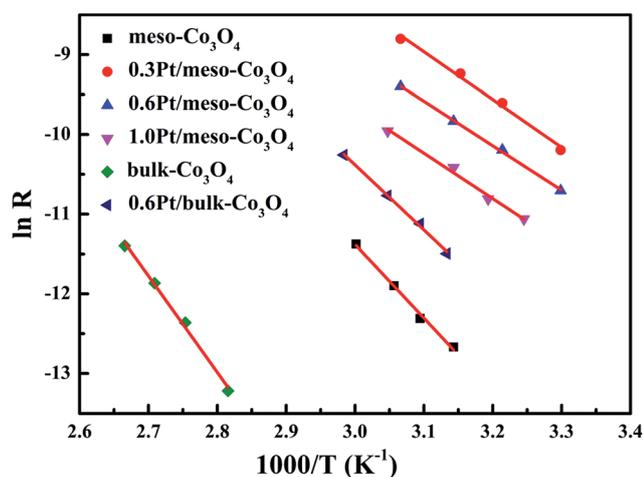
Fig. 11 Arrhenius plots in acetylene oxidation of meso-Co<sub>3</sub>O<sub>4</sub>, 0.3Pt/meso-Co<sub>3</sub>O<sub>4</sub>, 0.6Pt/meso-Co<sub>3</sub>O<sub>4</sub>, 1.0Pt/meso-Co<sub>3</sub>O<sub>4</sub>, bulk-Co<sub>3</sub>O<sub>4</sub> and 0.6Pt/bulk-Co<sub>3</sub>O<sub>4</sub>. Reaction gas composition: [C<sub>2</sub>H<sub>2</sub>] = 50 ppm, [O<sub>2</sub>] = 13 vol%, N<sub>2</sub> balance and GHSV = 30 000 h<sup>-1</sup>.
