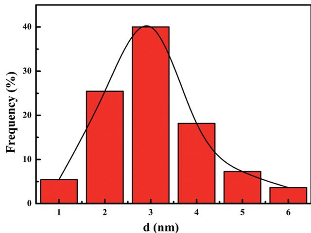
Fig. 4 Pt particles size distribution of 1.0Pt/meso- $\text{Co}_3\text{O}_4$ .
