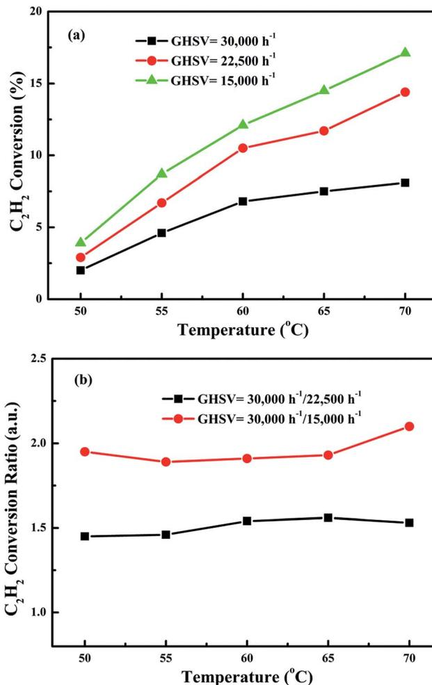
Fig. 9 (a) Acetylene conversion as a function of reaction temperature over meso-Co<sub>3</sub>O<sub>4</sub> at space velocities of 15 000 h<sup>-1</sup>, 22 500 h<sup>-1</sup> and 30 000 h<sup>-1</sup> and (b) acetylene conversion ratios for 15 000 h<sup>-1</sup>, 22 500 h<sup>-1</sup> and 30 000 h<sup>-1</sup> as a function of reaction temperature, using data from (a).
