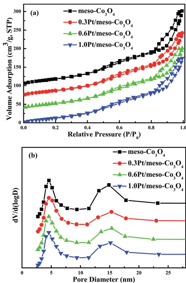
Fig. 1 (a) N<sub>2</sub> adsorption–desorption and (b) pore size distributions of meso-Co<sub>3</sub>O<sub>4</sub>, 0.3Pt/meso-Co<sub>3</sub>O<sub>4</sub>, 0.6Pt/meso-Co<sub>3</sub>O<sub>4</sub> and 1.0Pt/meso-Co<sub>3</sub>O<sub>4</sub>.
