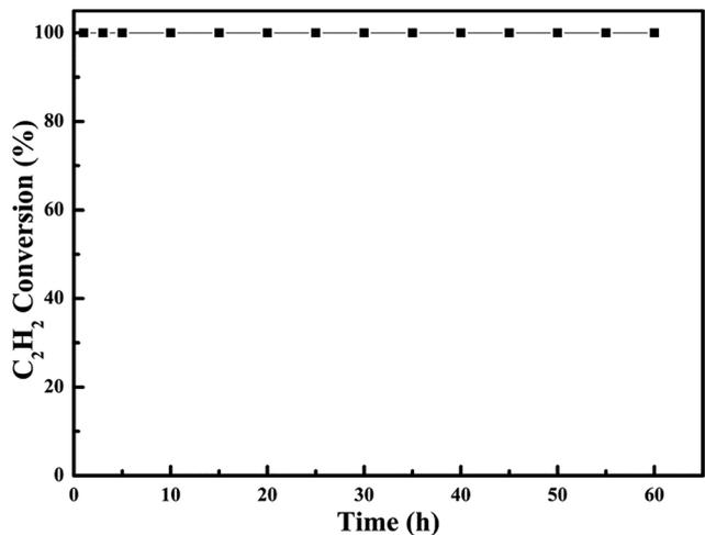
Fig. 13 Durability test on 0.6Pt/meso-Co<sub>3</sub>O<sub>4</sub> catalyst. Reaction gas composition: [C<sub>2</sub>H<sub>2</sub>] = 50 ppm, [O<sub>2</sub>] = 13 vol%, N<sub>2</sub> balance and GHSV = 30 000 h<sup>-1</sup>.
