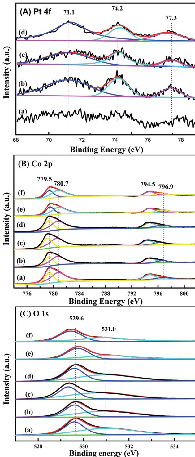
Fig. 6 (A) Pt 4f XPS spectra of (a) 0.3Pt/meso- $\text{Co}_3\text{O}_4$ , (b) 0.6Pt/meso- $\text{Co}_3\text{O}_4$ , (c) 1.0Pt/meso- $\text{Co}_3\text{O}_4$  and 0.6Pt/bulk- $\text{Co}_3\text{O}_4$ . (B) O 1s and (C) Co 2p XPS spectra of (a) meso- $\text{Co}_3\text{O}_4$ , (b) 0.3Pt/meso- $\text{Co}_3\text{O}_4$ , (c) 0.6Pt/meso- $\text{Co}_3\text{O}_4$ , (d) 1.0Pt/meso- $\text{Co}_3\text{O}_4$ , (e) bulk- $\text{Co}_3\text{O}_4$  and (f) 0.6Pt/bulk- $\text{Co}_3\text{O}_4$ .
