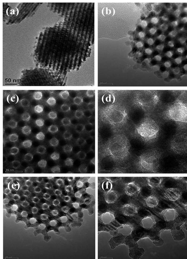
Fig. 3 TEM images of (a) meso- $\text{Co}_3\text{O}_4$ , (b) 0.3Pt/meso- $\text{Co}_3\text{O}_4$ , (c and d) 0.6Pt/meso- $\text{Co}_3\text{O}_4$  and (e and f) 1.0Pt/meso- $\text{Co}_3\text{O}_4$ .
