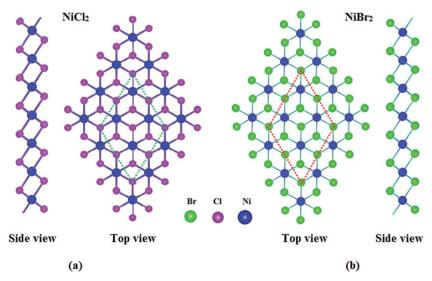
Fig. 1 Optimized geometric structures of (a) NiCl<sub>2</sub> and (b) NiBr<sub>2</sub> sheets. The selected  $2 \times 2$  supercell is marked by the dotted lines.
