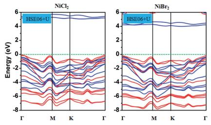
Fig. 4 Spin-polarized HSE06 + U band structures of  $NiCl_2$  and  $NiBr_2$  sheets. The red and blue solid lines correspond to the spin-up and spin-down states.
