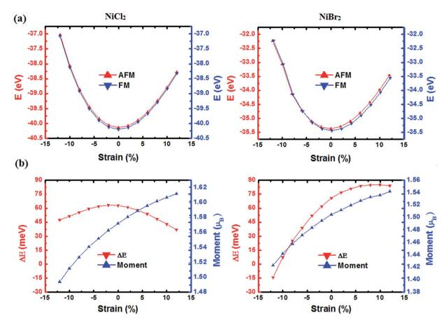
Fig. 6 (a) Change of total energies of ferromagnetic and antiferromagnetic NiCl<sub>2</sub> and NiBr<sub>2</sub> sheets with strain. (b) The changes of energy difference between AFM and FM couplings and magnetic moment of Ni atom with strain for NiCl<sub>2</sub> and NiBr<sub>2</sub> sheets.
