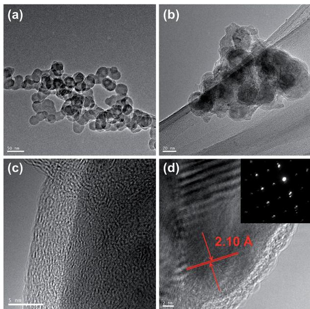
Fig. 3 TEM images of (a) Cu@Sn@PANI precursors and (b) resultant Cu<sub>6</sub>Sn<sub>5</sub>@C nanospheres. (c) HRTEM image and (d) SAED patterns of Cu<sub>6</sub>Sn<sub>5</sub>@C. Scale bars are 50, 20, 5, and 2 nm separately.
