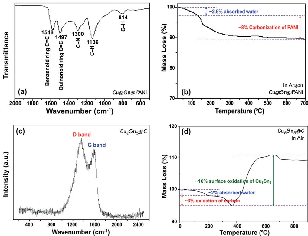
Fig. 2 (a) FTIR spectrum and (b) TGA curve in Ar of Cu@Sn@PANI precursors; (c) Raman spectrum and (d) TGA curve in air of Cu<sub>6</sub>Sn<sub>5</sub>@C nanospheres.
