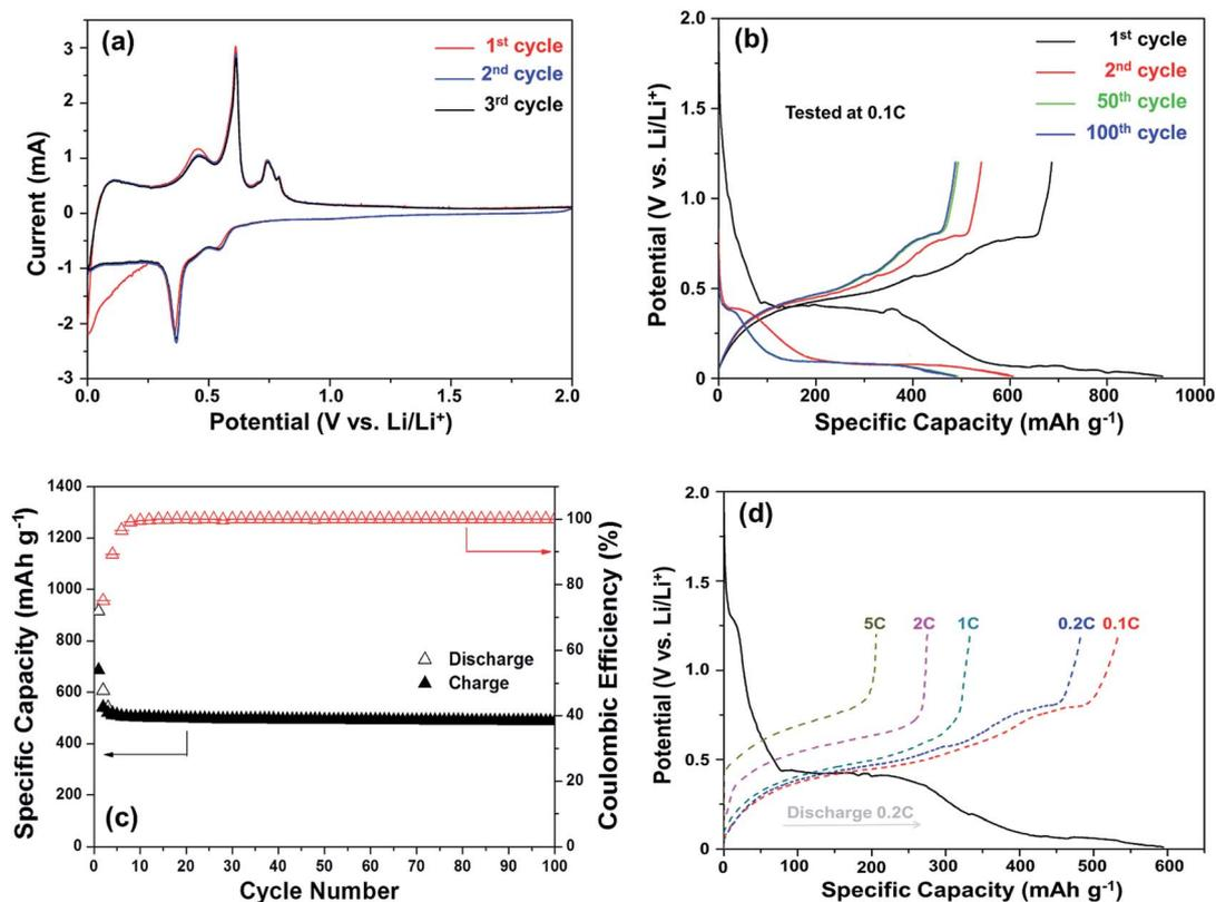
Fig. 4 Electrochemical performances of Li/Cu<sub>6</sub>Sn<sub>5</sub>@C cells: (a) CV curves at a scan rate of 0.1 mV s<sup>-1</sup>, (b) charge/discharge profiles at 0.1C (1C = 605 mA g<sup>-1</sup>), (c) the cycleability and coulombic efficiency at 0.1C, and (d) high-rate performances.
