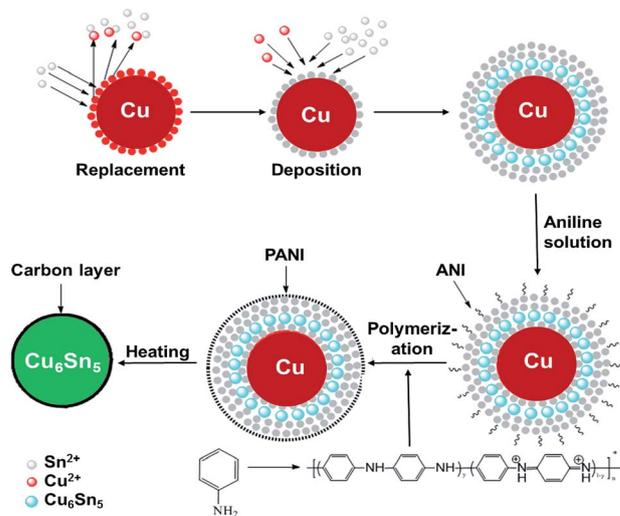
Scheme 1 Schematic of the preparation of the core-shell Cu<sub>6</sub>Sn<sub>5</sub>@C nanospheres.
