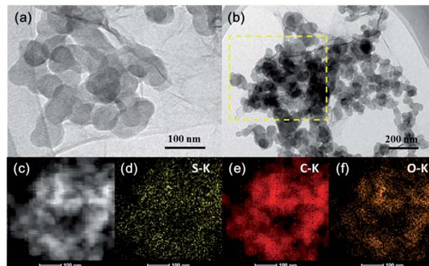
Fig. 2 TEM images of GO-PEG@C/S with a scale bar of (a) 100 nm and (b) 200 nm; (c) HAADF-STEM image of the yellow dotted area in (b), and the corresponding elemental mapping of (d) sulfur, (e) carbon and (f) oxygen.
