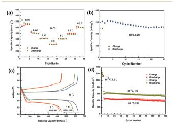
Fig. 6 The GO-PEG@C/S material-based all-solid-state Li-S battery at 80 °C and (a) different rates and (b) 0.2C. (c) Discharge/charge curves and (d) cycling performance of the GO-PEG@C/S materialbased all-solid-state Li-S battery at 1C or 2C and 80 °C. The capacity is calculated based on the mass of sulfur in the electrode
