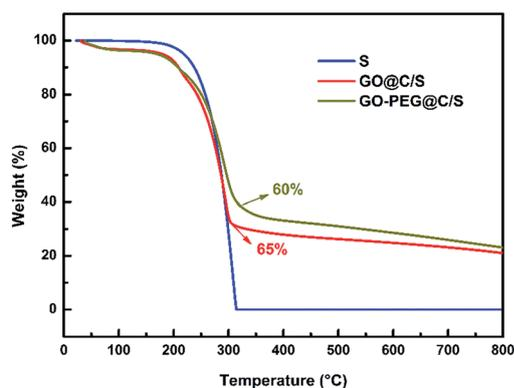
Fig. 4 Thermogravimetric curves of sublimed sulfur, GO@C/S and GO-PEG@C/S materials.
