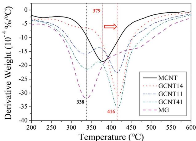
Fig. 6 DTG curves of MCNT, GCNT14, GCNT11, GCNT41 and MG.
