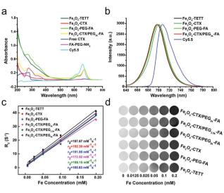
Fig. 2 UV-Vis absorbance (a) and fluorescence emission (b) spectra,  $r_2$  relaxivities (c), and the corresponding MR  $T_2$ -weighted MR mapping (d) of NPs.
