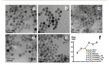
Fig. 1 TEM images of Fe $_3$ O $_4$ -CTX (a), Fe $_3$ O $_4$ -PEG-FA (b), Fe $_3$ O $_4$ -CTX/PEG $_{2k}$ -FA (c), Fe $_3$ O $_4$ -CTX/PEG $_{3.5k}$ -FA (d), and Fe $_3$ O $_4$ -CTX/PEG $_{5k}$ -FA (e) NPs, and their DLS sizes (f).
