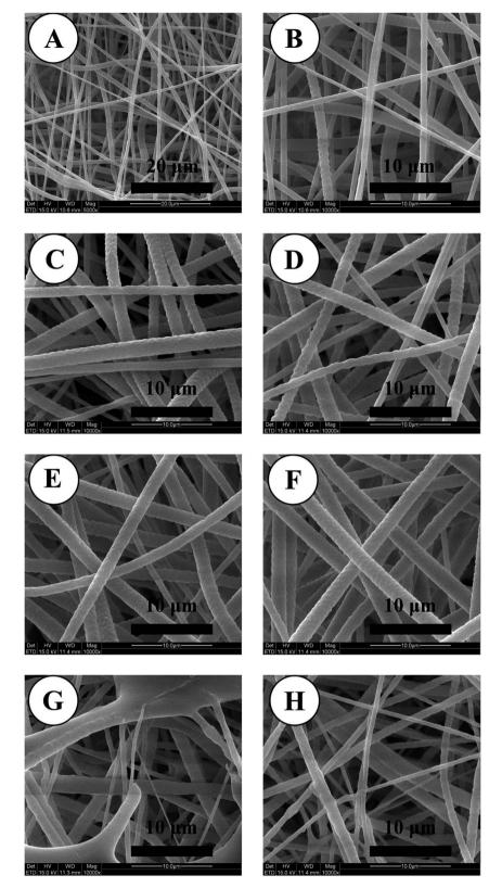
Fig. 1 Micromorphology of electrospun nanofibrous mats before and after the deposition of the polyelectrolytes (SEM images). (A and B) PCL; (C) PCL-(PEI/Hep)<sub>5</sub>; (D) PCL-(SePEI/Hep)<sub>10</sub>; (F) PCL-(SePEI/Hep)<sub>10</sub>; (G) PCL-(PEI/Hep)<sub>15</sub>; (H) PCL-(SePEI/Hep)<sub>15</sub>.
