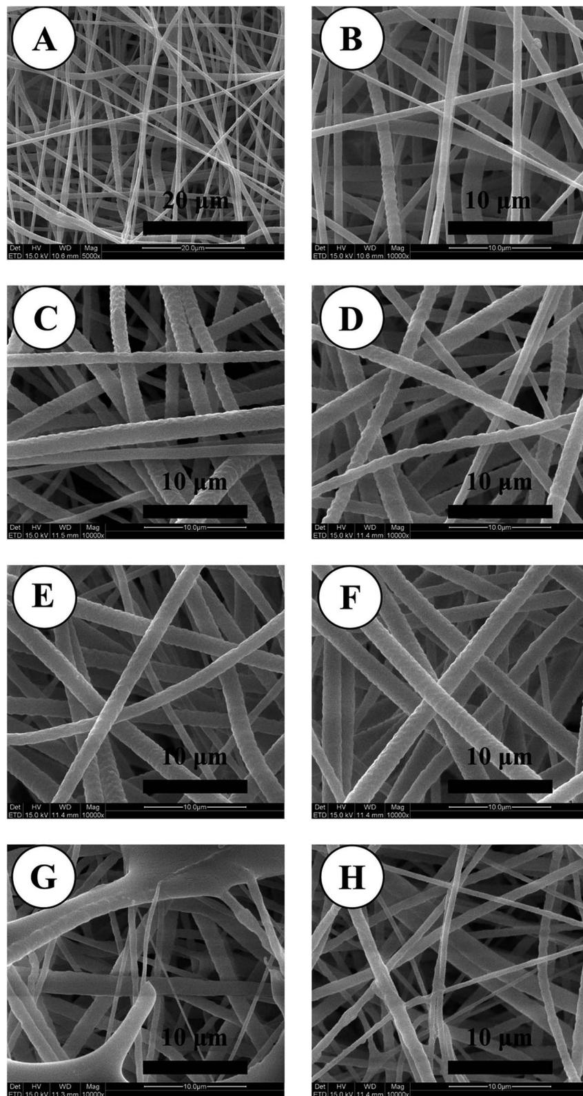
Fig. 1 Micromorphology of electrospun nanofibrous mats before and after the deposition of the polyelectrolytes (SEM images). (A and B) PCL; (C) PCL-(PEI/Hep)<sub>5</sub>; (D) PCL-(SePEI/Hep)<sub>5</sub>; (E) PCL-(PEI/Hep)<sub>10</sub>; (F) PCL-(SePEI/Hep)<sub>10</sub>; (G) PCL-(PEI/Hep)<sub>15</sub>; (H) PCL-(SePEI/Hep)<sub>15</sub>.
