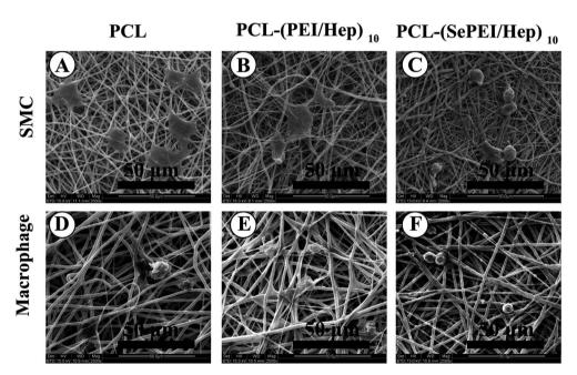
Fig. 5 Morphology of SMCs and macrophages on different samples (scale bar: 50 μm).
