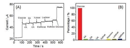
Fig. 8 (A) Interference test for Ni(OH)<sub>2</sub>/ECF-0.06 modified electrode in 0.1 M NaOH at +0.55 V with 1.0 mM glucose and other interferents, including AA, DA, UA, xylose, mannose, lactose, and maltose (all 0.1 mM). (B) Interfering signal percentages compared with glucose.
