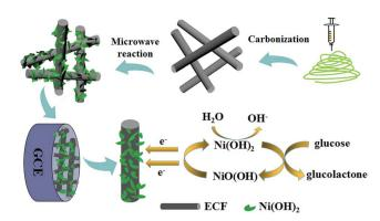
Scheme 1 Construction procedure for Ni(OH)<sub>2</sub>/ECF sensor.
