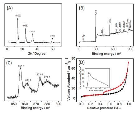
Fig. 3 (A) XRD pattern, (B) XPS survey spectrum, (C) high-resolution Ni 2p spectrum, and (D) nitrogen adsorption—desorption isotherms of Ni(OH)<sub>2</sub>/ECF-0.06 hybrid. Inset: pore size distribution calculated using the Barrett–Joyner–Halenda (BJH) method.
