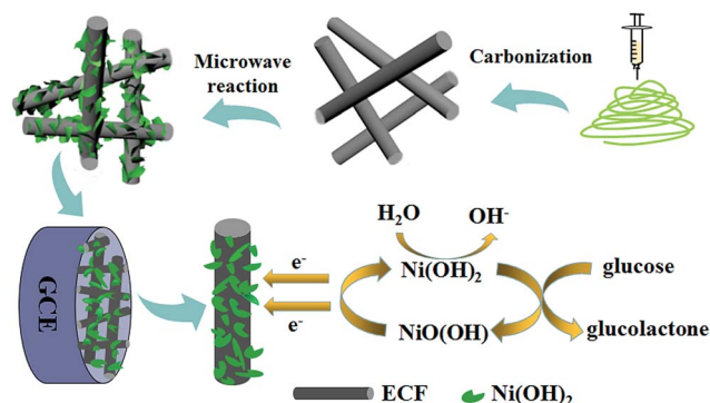
Scheme 1 Construction procedure for Ni(OH) 2 /ECF sensor.
