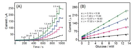
Fig. 7 (A) Amperometric responses of (a) pure  $Ni(OH)_2$  nanoplatelet modified electrodes, (b)  $Ni(OH)_2/ECF-0.03$ , (c)  $Ni(OH)_2/ECF-0.06$  and (d)  $Ni(OH)_2/ECF-0.12$  upon successive addition of different glucose concentrations to 0.1 M NaOH solution at +0.55 V. (B) Plots of current *versus* corresponding glucose concentration.
