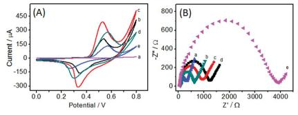
Fig. 4 (A) CV curves and (B) Nyquist plots of (a) ECF, (b)  $Ni(OH)_2/ECF-0.03$ , (c)  $Ni(OH)_2/ECF-0.06$ , (d)  $Ni(OH)_2/ECF-0.12$  and (e) pure  $Ni(OH)_2$  nanoplatelets in 0.1 M NaOH solution, using a scan rate of 50 mV s<sup>-1</sup>.
