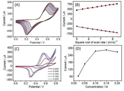
Fig. 6 (A) CV curves of Ni(OH)<sub>2</sub>/ECF-0.06 at different scan rates from 25 to 70 mV s<sup>-1</sup> (inside to outside: 25 to 70 mV s<sup>-1</sup>) in 0.1 M NaOH solution and (C) in NaOH concentrations of 0.02–0.20 M containing 2.0 mM glucose. (B) Plots of anodic and cathodic peak currents *versus* the square root of the scan rate. (D) Calibration curves of peak current *versus* NaOH concentration.
