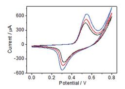
Fig. 5 CV curves of Ni(OH)<sub>2</sub>/ECF-0.06 modified electrode in 0.1 M NaOH solution containing glucose concentrations of 50  $\mu$ M (black line), 100  $\mu$ M (red line), and 200  $\mu$ M (blue line) at a scan rate of 50 mV s<sup>-1</sup>.
