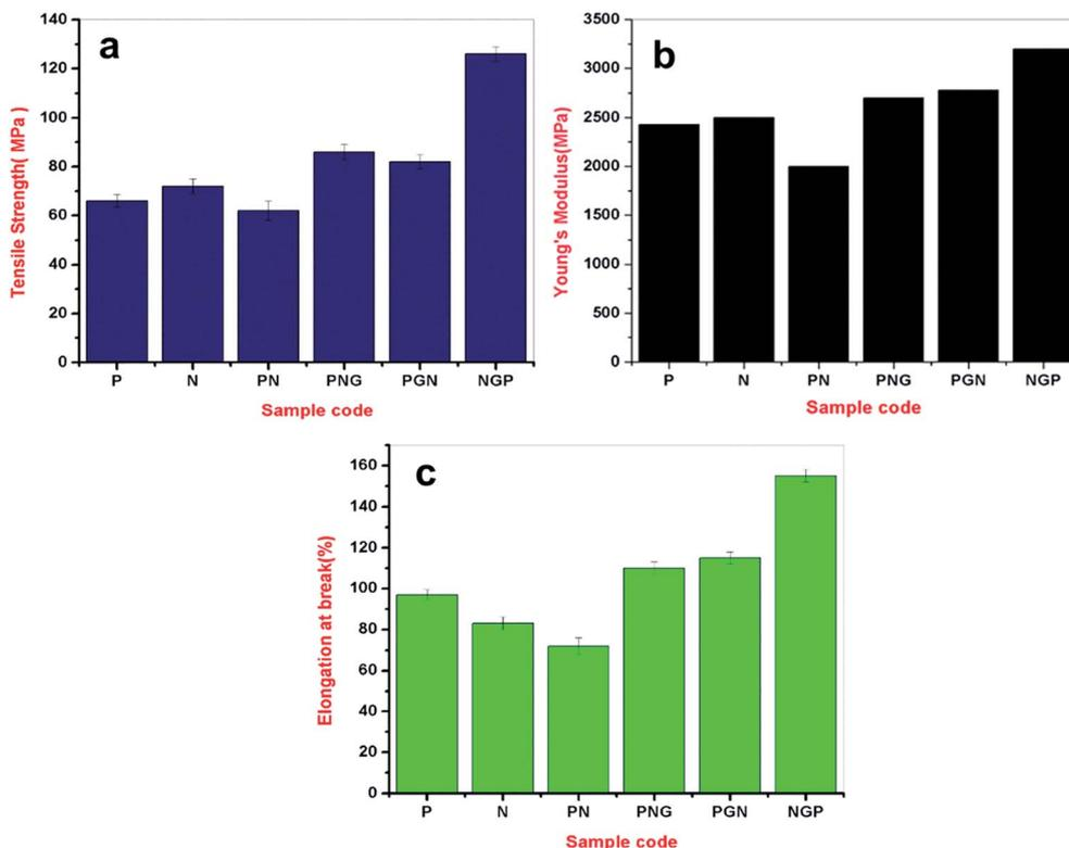
Fig. 10 Tensile modulus, Young modulus and elongation at break of the prepared nanocomposites along with pure polymers.
