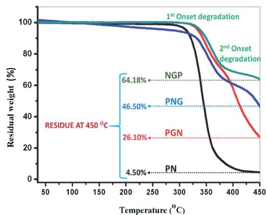
Fig. 4 TGA plot showing 1<sup>st</sup> and 2<sup>nd</sup> onset degradation and corresponding weight loss of prepared neat blend and PNCs.
