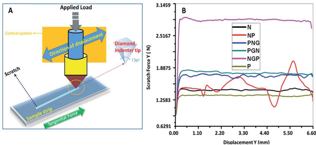
Fig. 6 (A) Schematic diagram showing scratch hardness and depth indentation testing and (B) depth profile results of a typical scratch on surface on the strip surface of pure polymers and prepared composites.
