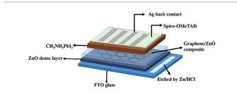
Fig. 1 Schematic of the perovskite solar cell architecture fabricated using G/ZnO nanocomposite as an electron transporting layer.
