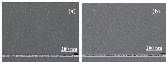
Fig. 3 SEM images of (a) ZnO and (b) 0.75 wt% G/ZnO nano-composite films.
