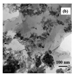
Fig. 5 TEM images of (a) graphene, (b) G/ZnO nanocomposite and inset of (a) shows the Raman spectrum of graphene.
