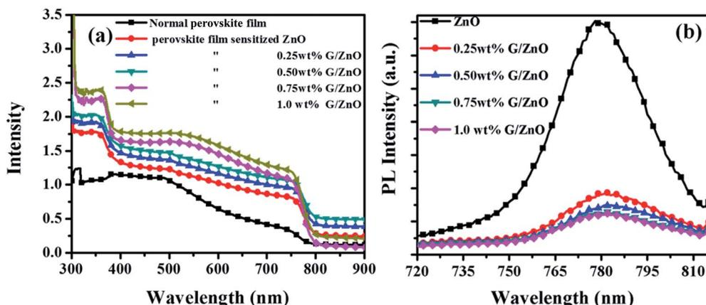
Fig. 6 (a) Absorbance and (b) photoluminescence spectra of perovskite films on G/ZnO nanocomposites with different graphene concentration.
