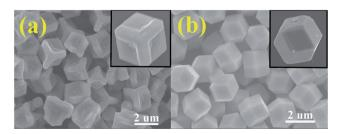
Fig. 2 SEM images of (a) Ag<sub>3</sub>PO<sub>4</sub> CRD and (b) Ag<sub>3</sub>PO<sub>4</sub> RD.
