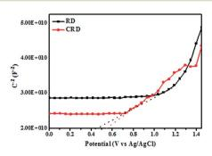
Fig. 6 Mott-Schottky plots of Ag<sub>3</sub>PO<sub>4</sub> CRD and Ag<sub>3</sub>PO<sub>4</sub> RD.
