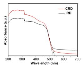
Fig. 4 UV-Vis absorption spectra of Ag<sub>3</sub>PO<sub>4</sub> CRD and Ag<sub>3</sub>PO<sub>4</sub> RD.
