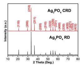
Fig. 1 XRD patterns of Ag<sub>3</sub>PO<sub>4</sub> CRD and Ag<sub>3</sub>PO<sub>4</sub> RD.
