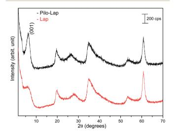
Fig. 4 XRD patterns of powdered Lap (red line) and Pilo-Lap (black line).
