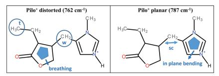
Schematic representation of the vibrational modes of Pilo<sup>+</sup> distorted at 762 cm<sup>-1</sup> and Pilo<sup>+</sup> planar at 787 cm<sup>-1</sup>.
