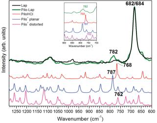
Fig. 6 Experimental FT-Raman spectra obtained for Lap (black line), Pilo-Lap (green line) and PiloHCl (red line). Theoretical spectra obtained for Pilo<sup>+</sup> planar (blue line) and Pilo<sup>+</sup> distorted (pink line). Inset: zoom of the region between 700 and 900  $\mbox{cm}^{-1};$  the Lap line has been omitted
