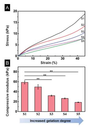
Fig. 7 Mechanical properties of SF/agarose scaffolds in wet conditions. (A) Compressive strain-stress curves of scaffolds. (B) Compression modulus of scaffolds. Data are shown as mean  $\pm$  standard deviation, n = 3 (\*\* $p \le 0.01$ ).
