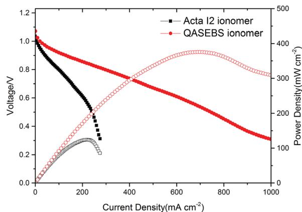
Fig. 5 The cell performance of the different electrode with the Acta I2 ionomer and QASEBS ionomer. Test conditions: cell and  $\text{H}_2/\text{O}_2$  temperatures of  $50^\circ\text{C}$ ; flow rates of  $0.1\text{ L min}^{-1}$  and  $0.2\text{ L min}^{-1}$  for  $\text{H}_2$  and  $\text{O}_2$ , respectively; and back pressure of  $200\text{ kPa}$  for  $\text{H}_2$  and  $\text{O}_2$ .
