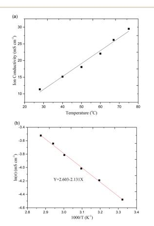
Fig. 3 Ionic conductivity (a) and Arrhenius plot (b) of the QASEBS with  ${\rm OH^-}$  form at different temperatures.
