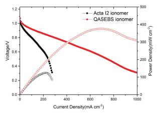
Fig. 5 The cell performance of the different electrode with the Acta I2 ionomer and QASEBS ionomer. Test conditions: cell and H2/O2 temperatures of 50 °C; flow rates of 0.1 L min<sup>-1</sup> and 0.2 L min<sup>-1</sup> for H<sub>2</sub> and O2, respectively; and back pressure of 200 kPa for H2 and O2.
