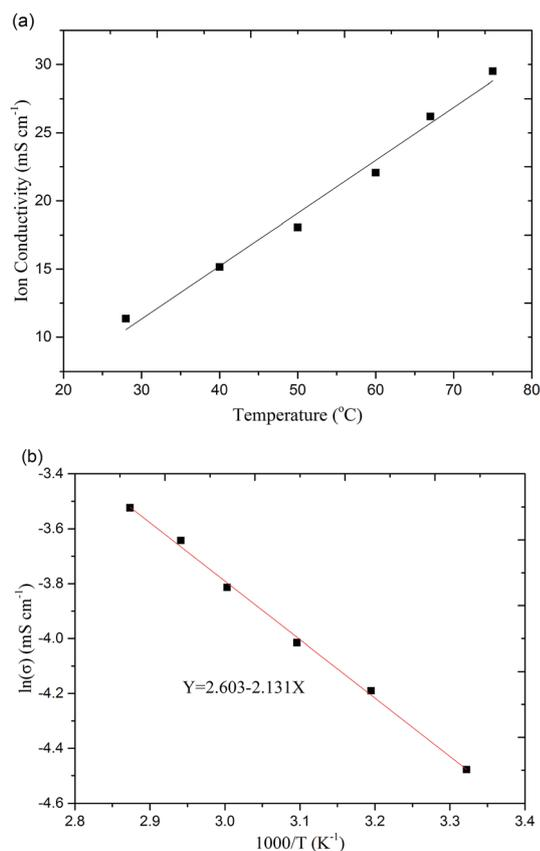
**Fig. 3** Ionic conductivity (a) and Arrhenius plot (b) of the QASEBS with OH<sup>-</sup> form at different temperatures.
