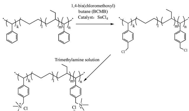
Scheme 1 The synthetic procedure of the quaternary ammonium SEBS block copolymer in Cl<sup>-</sup> form.
