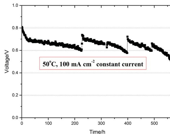
**Fig. 7** Durability test for MEA with QASEBS ionomer. Test conditions: constant current density 100 mA cm<sup>-2</sup>, cell and H<sub>2</sub>/O<sub>2</sub> temperatures of 50 °C; flow rates of 0.1 L min<sup>-1</sup> and 0.2 L min<sup>-1</sup> for H<sub>2</sub> and O<sub>2</sub>, respectively; and back pressure of 200 kPa for H<sub>2</sub> and O<sub>2</sub>.
