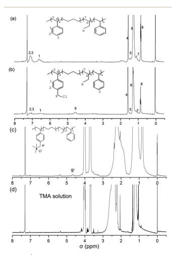
Fig. 1 (a) <sup>1</sup>H NMR spectra of Asahi KASE Tuftec SEBS H1031, (b) CMSEBS, (c) QASEBS (Cl type) and (d) TMA solution in chloroform-d.
