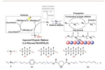
Scheme 1 Proposed polymerization mechanism of photo-induced step tranfer-addition  $\vartheta$  radical-termination (START) strategy in aqueous/organic biphase.
