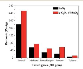
Fig. 11 Comparison of the response values of the pure  $SnO_2$  and the  $g-C_3N_4-5P/SnO_2$  composite sensors to 500 ppm different gases at 300 °C.
