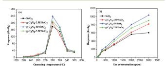
Fig. 9 The response values of the SnO $_2$ , g-C $_3$ N $_4$ -2.5P/SnO $_2$ , g-C $_3$ N $_4$ -5P/SnO $_2$  and g-C $_3$ N $_4$ -7.5P/SnO $_2$  to 500 ppm ethanol (a) under different operating temperature, (b) for different concentrations of ethanol at 300 °C.
