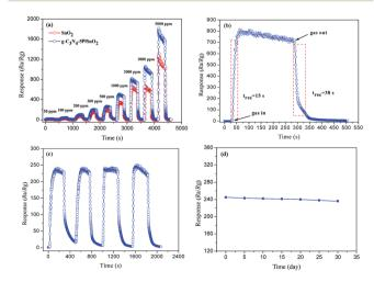
Fig. 10 (a) Real time response curves of the pure  $SnO_2$  and  $g-C_3N_4-5P/SnO_2$  composite sensors to ethanol in the range of 50-5000 ppm, (b) response–recovery time characteristics of the  $g-C_3N_4-5P/SnO_2$  composite sensor to 2000 ppm ethanol at 300 °C, (c) repeatability and (d) stability behaviors of the  $g-C_3N_4-5P/SnO_2$  composite sensor to 500 ppm ethanol at 300 °C.
