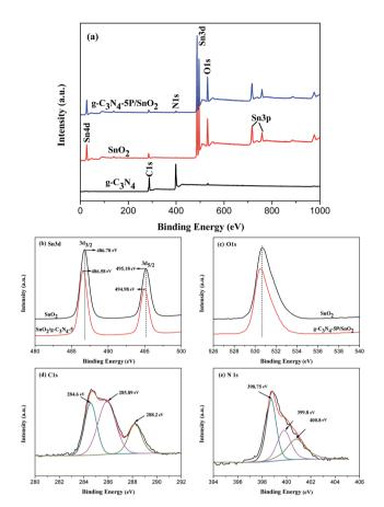
Fig. 8 XPS survey of  $g-C_3N_4$ ,  $SnO_2$  and  $g-C_3N_4-5P/SnO_2$  samples: (a) the general scan spectrum, (b) Sn 3d spectrum, (c) O 1s spectrum, (d) C 1s spectrum, and (e) N 1s spectrum.
