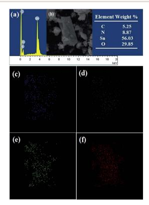
Fig. 5 (a) EDS spectra of the  $g-C_3N_4-5P/SnO_2$  composite, (b) SEM image and elements content for selected EDS area, and EDS mappings of C (c), N (d), O (e), Sn (f) element related to (b).
