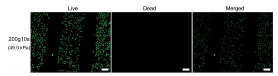
Fig. 7 Live/dead assay to evaluate cell viability of A549 on PLGA electrospun nanofiber sheets after cell micropatterning process. A549 cells were pressed for 10 s under the pressure of 49.0 kPa (a weight of 200 g was used). The scale bars are 100 μm.
