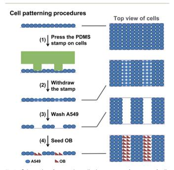
Fig. 1 Schematics of generating cell micropatterns of one type of cells and di-cell co-culture micropatterns using  $\mu$ -eraser strategy.
