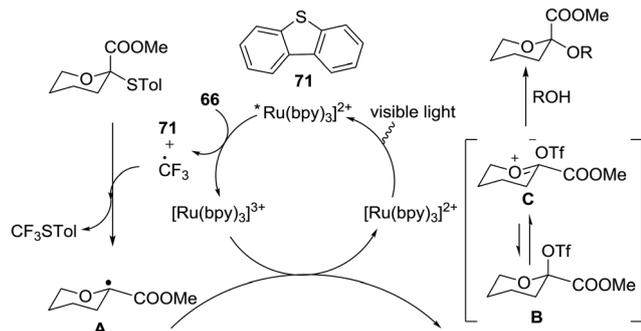
Fig. 14 Proposed mechanism for visible light photoredox-catalyzed O-sialylation.
