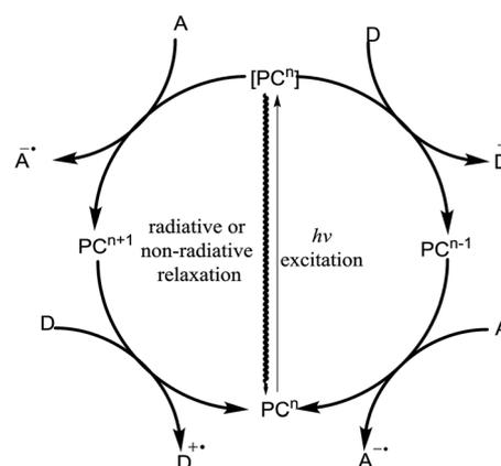
Fig. 5 General cycle for photoinduced electron transfer (PET).
