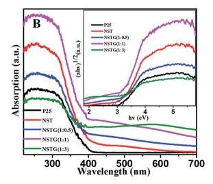
Fig. 5 (A) UV-vis absorption spectrum of N, S-GQDs and inset shows images of the different colors of N, S-GQD. (B) UV-vis absorption spectra of P25, NST, NSTG(1:0.5), NSTG(1:1), and NSTG(1:3). The inset is the estimated band gap from the Kubelka–Munk function.
