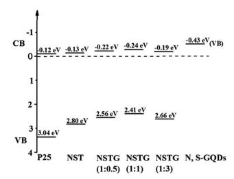
Scheme 1 Schematic illustration of the DOS of NSTG(1: 0.5), NSTG(1: 1), NSTG(1: 3), and N, S-GQDs.
