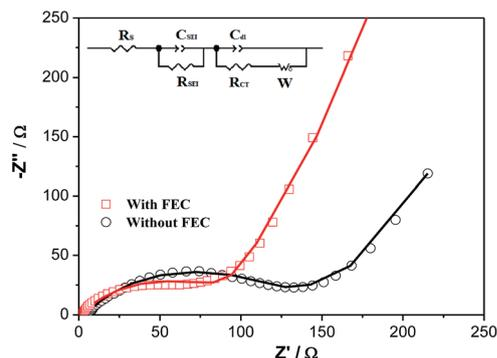
Fig. 8 Electrochemical impedance spectra of the Li/ZnCo<sub>2</sub>O<sub>4</sub> cells in the electrolytes with and without FEC after 200 cycles. The squares and circles are the experimental data and the curves are the fitted results of the experimental data using the equivalent circuit given in the inset.
