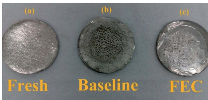
Fig. 9 Images of the pristine lithium electrode (a) and the lithium electrodes of the Li/ZnCo<sub>2</sub>O<sub>4</sub> cells in the electrolytes without (b) and with (c) FEC after 200 cycles.
