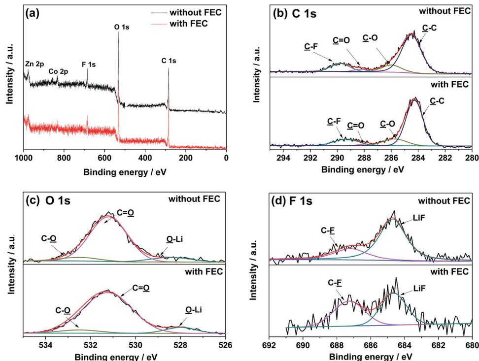
Fig. 7 (a) XPS survey spectra of the  $\text{ZnCo}_2\text{O}_4$  electrodes cycled in the electrolyte with and without FEC. (b) Deconvoluted C 1s, (c) deconvoluted O 1s, and (d) deconvoluted F 1s spectra of the  $\text{ZnCo}_2\text{O}_4$  electrodes cycled in the electrolyte with and without FEC.
