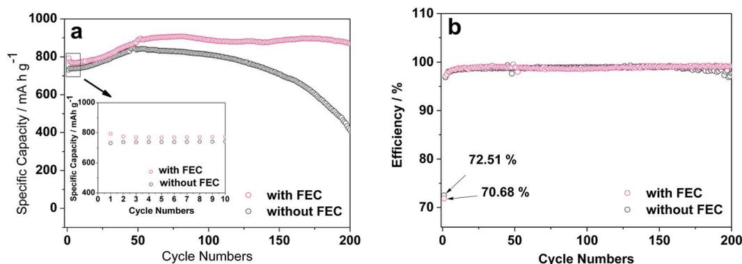
Fig. 1 Cycling performance (a) and coulombic efficiency (b) of the Li/ZnCo<sub>2</sub>O<sub>4</sub> cells in the electrolytes with and without FEC at the current density of 200 mA g<sup>-1</sup>. Cycling performance of the Li/ZnCo<sub>2</sub>O<sub>4</sub> cells in the electrolytes with and without FEC at the first 10 cycles is shown in (a).
