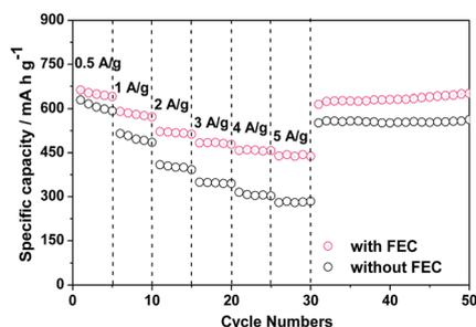
Fig. 2 Rate capacities of the Li/ZnCo<sub>2</sub>O<sub>4</sub> cells in the electrolytes with and without FEC.
