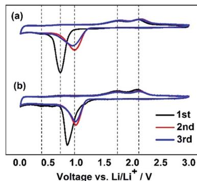
Fig. 4 CV curves of the Li/ZnCo<sub>2</sub>O<sub>4</sub> cells in the electrolyte without (a) and with (b) FEC.
