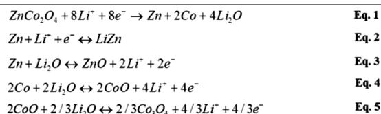
Fig. 3 Electrochemical reactions associated with the discharge and charge processes of the ZnCo<sub>2</sub>O<sub>4</sub> based anode in LIBs.
