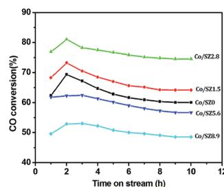
Fig. 7 The time-on-stream CO conversion of Co/SZ catalyst.
