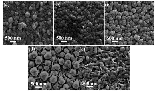
Fig. 6 (a-e) Surface morphology of  $CoSb_3$  thin films deposited at -0.8 V, -0.9 V, -0.9 V, -1.0 V, and -1.1 V deposition potentials respectively. It is clearly noticeable that first the globular grains increase in size attaining near uniform sizes as deposition potential reaches -0.97 V, and thereafter flake-like grains start forming with increasing number density.
