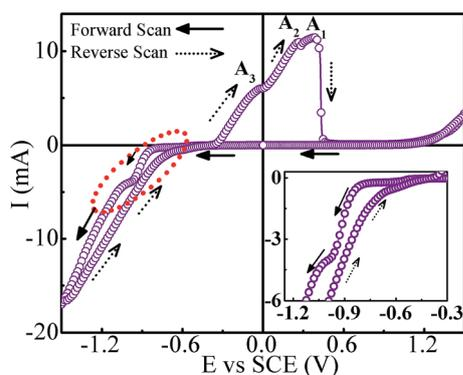
Fig. 3 Cyclic voltammogram for Co–Sb deposition from pH  $\sim 3$  electrolyte bath consisting of  $0.003 \text{ M Sb}_2\text{O}_3$ ,  $0.172 \text{ M CoSO}_4 \cdot 7\text{H}_2\text{O}$ ,  $0.125 \text{ M}$  sodium citrate and  $0.196 \text{ M}$  citric acid (inset shows the zoomed view of cathodic scan).
