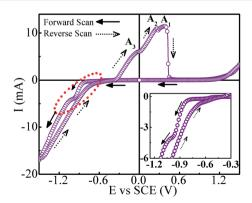
Fig. 3 Cyclic voltammogram for Co–Sb deposition from pH  $\sim$ 3 electrolyte bath consisting of 0.003 M Sb<sub>2</sub>O<sub>3</sub>, 0.172 M CoSO<sub>4</sub>·7H<sub>2</sub>O, 0.125 M sodium citrate and 0.196 M citric acid (inset shows the zoomed view of cathodic scan).
