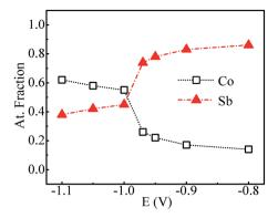
Fig. 4 Atomic% of Co and Sb in samples prepared at various deposition potentials.
