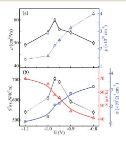
Fig. 10 (a) Hole carrier concentration and Hall mobility variation, and (b) power factor, Seebeck coefficient and electrical conductivity variation of CoSb<sub>3</sub> thin films as a function of deposition potential (lines serve as guide to the eye). The error bars in the data points show the variation in values obtained for three sets of samples prepared under similar conditions.
