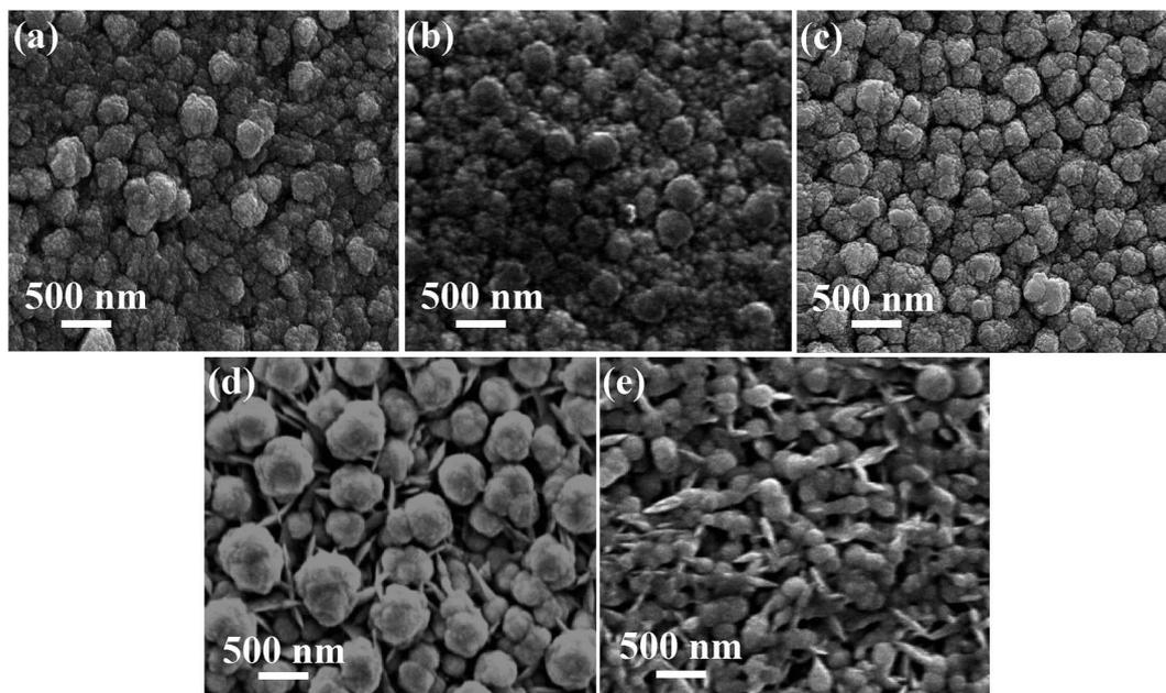
Fig. 6 (a–e) Surface morphology of  $\text{CoSb}_3$  thin films deposited at  $-0.8$  V,  $-0.9$  V,  $-0.97$  V,  $-1.0$  V, and  $-1.1$  V deposition potentials respectively. It is clearly noticeable that first the globular grains increase in size attaining near uniform sizes as deposition potential reaches  $-0.97$  V, and thereafter flake-like grains start forming with increasing number density.
