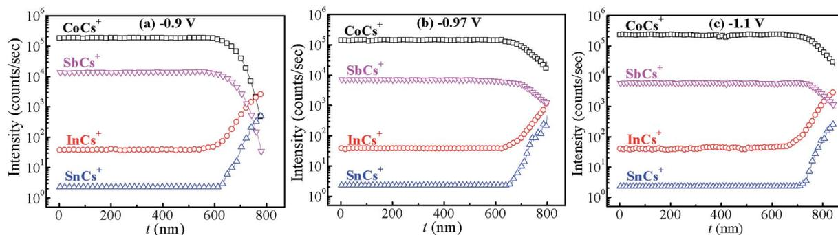
Fig. 5 SIMS depth profiles recorded on the films prepared at different deposition potentials (a)  $-0.9$  V, (b)  $-0.97$  V and (c)  $-1.1$  V. The signals corresponding to  $\text{InCs}^+$  and  $\text{SnCs}^+$  are from the underlying ITO substrate.
