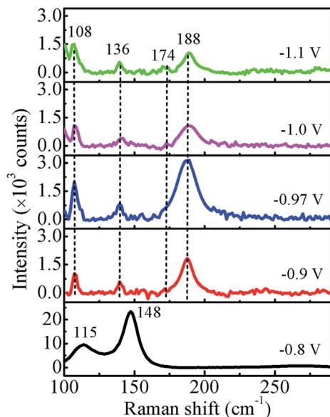
Fig. 9 Room temperature Raman spectra of CoSb<sub>3</sub> films deposited at different deposition potentials.
