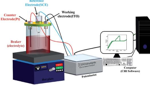
Fig. 1 Schematic of the electrodeposition set-up.
