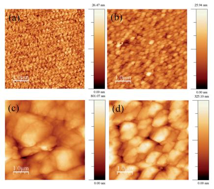
Fig. 2 Topographical images of (a) untreated ITO substrate, (b) treated ITO substrate, (c) CoSb<sub>3</sub> thin film on untreated ITO and (d) CoSb<sub>3</sub> thin film on treated ITO substrate.
