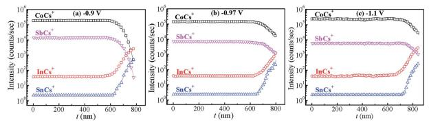
Fig. 5 SIMS depth profiles recorded on the films prepared at different deposition potentials (a) -0.9 V, (b) -0.97 V and (c) -1.1 V. The signals corresponding to InCs<sup>+</sup> and SnCs<sup>+</sup> are from the underlying ITO substrate.
