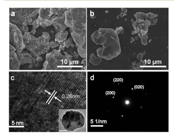
Fig. 3 (a) SEM image of binary FeS precursor. (b) SEM image, (c) high-resolution TEM image and (d) SAED pattern along the [001] zone axis of  $K_x(C_2H_8N_2)_yFe_{2-z}S_2$  with x=0.35. Inset of (c) shows the regular TEM image with the scaleplate as 2  $\mu$ m.
