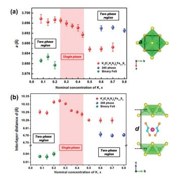
Fig. 2 (a) The lattice parameters a and (b) interlayer distances d of  $K_x(C_2H_8N_2)_yFe_{2-z}S_2$ , 245 phase and binary FeS depended on the nominal K concentration, x. The light red area shows the single-phase region of the intercalated phase. The structural model of  $C_2H_8N_2$  molecule was adopted from ref. 28.
