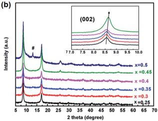
Fig. 1 (a) PXRD pattern of binary FeS and  $K_x(C_2H_8N_2)_yFe_{2-z}S_2$  (x=0.35), where the green and red vertical lines represent Bragg diffractions of I4/m and P4/nmm space groups, respectively. Inset shows the enlarged pattern of  $K_x(C_2H_8N_2)_yFe_{2-z}S_2$  from 30 to 60 2theta degree. (b) PXRD patterns of  $K_x(C_2H_8N_2)_yFe_{2-z}S_2$  with different x. Inset shows the enlarged (002) peaks. # represents the diffraction peak of 245 phase.
