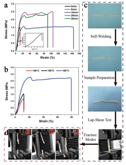
Fig. 7 The mechanical properties of the self-welded PUV-3 for (a) different time at 150 °C and (b) 5 min at different temperature. (c) Sample of the lap-shear test. (d) Fracture modes of the self-welded samples.
