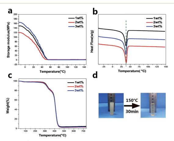
Fig. 2 (a) Storage modulus (E') vs. temperature curves of the PUVs. (b) Differential scanning calorimeter (DSC) curves of the PUVs. (c) Thermogravimetric analysis (TGA) of the PUVs in nitrogen atmosphere. (d) Melting experiment of the crosslinked PUV-3.
