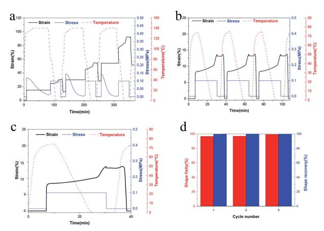
Fig. 5 (a) Consecutive elasticity/plasticity cycles. (b) Consecutive elasticity cycles. (c) A representative elasticity cycle. (d) Shape fixity ( $R_f$ ) and shape recovery ( $R_r$ ) ratio of the PUV-3 with the elasticity cycles.
