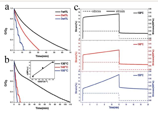
Fig. 3 (a) Stress relaxation behavior for various catalyst concentrations at 140 °C. (b) Stress relaxation of the PUV-3 at various temperatures. (c) Creep and recovery curves of the PUV-3 at different temperatures.
