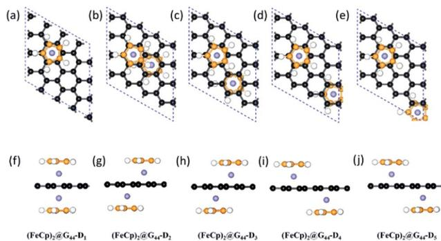
Fig. 4 (a–j) Top and side views of the optimized structures of  $(\text{FeCp})_2@G_{44-D_i}$ ,  $i = 1-5$ . Black and orange balls represent the carbon atoms of graphene and Cp ligands; and white and purple balls represent H and Fe atoms, respectively. The complete descriptions of  $(\text{FeCp})_2@G_{44-D_4}$  (c) and  $(\text{FeCp})_2@G_{44-D_5}$  (d) are depicted in the  $2 \times 2$  supercells in Fig. S1(c, d, g and f) in the ESI†
