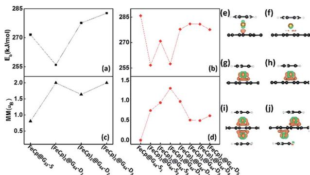
**Fig. 2** Binding energies (a and b) and total magnetic moments (c and d) of  $(\text{FeCp})_n@G_{33\text{S}}$  and  $(\text{FeCp})_n@G_{44\text{S}}$ ,  $n = 1, 2$ . CDD plots of  $\text{FeBz}@G_{33\text{-S}}$  (e),  $\text{FeBz}@G_{44\text{-S}}$  (f),  $\text{FeCp}@G_{33\text{-S}}$  (g),  $\text{FeCp}@G_{44\text{-S}}$  (h),  $(\text{FeCp})_2@G_{33\text{-D}}_1$  (i) and  $(\text{FeCp})_2@G_{33\text{-D}}_2$  (j).
