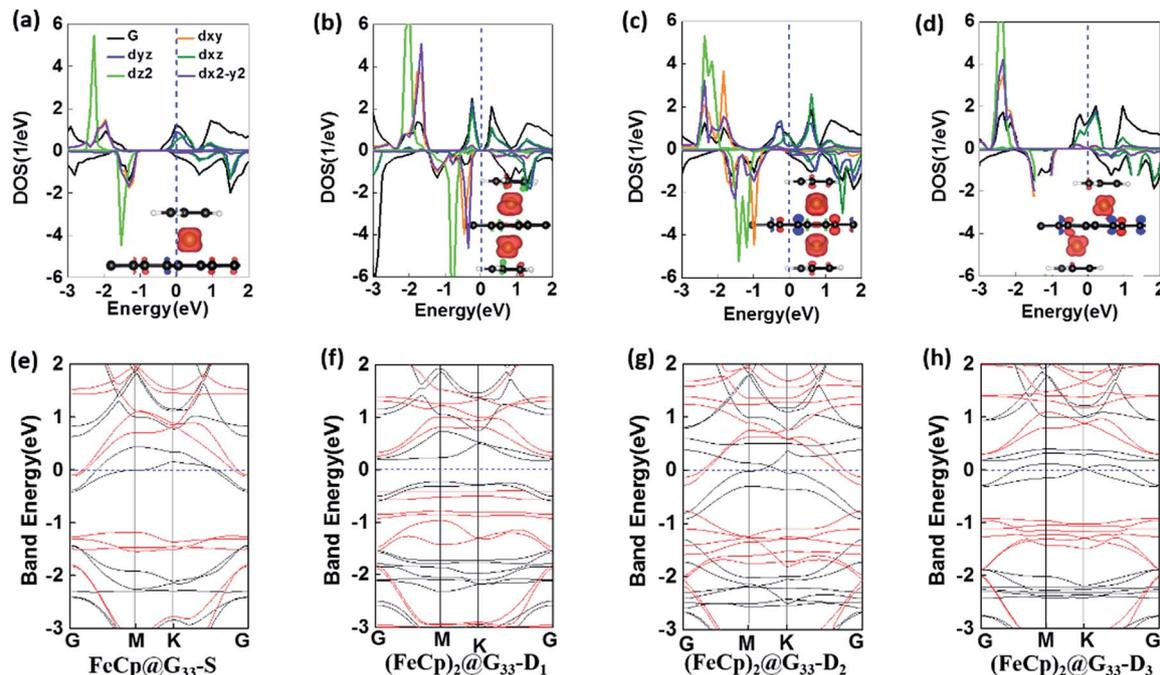
Fig. 3 (a–d) Projected density of states (DOS) and (e–h) electronic band structures of  $(\text{FeCp})_n@G_{33S}$ ,  $n = 1, 2$ . The black and red lines correspond to the spin-up and spin-down channels, respectively. Insets are the spin densities plots.
