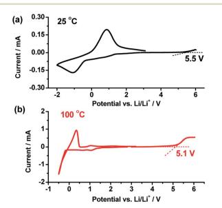
Fig. 4 Linear sweep and cyclic voltammetry results at (a) 25 °C and (b) 100 °C. The negative scan OCV  $\rightarrow$  -2 V  $\rightarrow$  OCV and OCV  $\rightarrow$  -0.5 V  $\rightarrow$  OCV at respectively 25 °C and 100 °C, and the positive scan OCV  $\rightarrow$ 6 V at a rate of 10 mV s<sup>-1</sup> were conducted.
