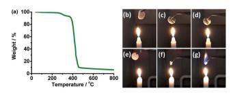
Fig. 3 Thermal stability characterization of the wheat flour modified SPE. (a) Thermal analysis of the SPE. The SPE (b) was placed close to the flame, the electrolyte at (c) and (d) were still self-standing after 10 seconds. As a comparison, the Celgard separator with liquid organic electrolyte (e) was also placed close to the flame and stopped at almost the same position with SPE, (f) the separator shrunk in less than 1 second and (g) the electrolyte burned.
