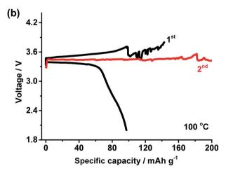
Fig. 6 (a) Charge/discharge curves of PEO + LiTFSI and PEO + LiTFSI + wheat flour based LiFePO $_4$  battery at 25  $^{\circ}$ C and (b) charge/discharge curves of PEO + LiTFSI based LiFePO $_4$  battery at 100  $^{\circ}$ C and 1C.
