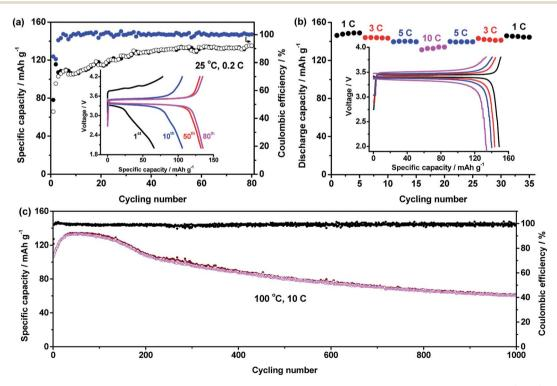
Fig. 5 Cycling performance of LiFePO<sub>4</sub>/SPE/Li battery at (a) 25 °C and 0.2C, inset is the charge/discharge curve at 1<sup>st</sup>, 10<sup>th</sup>, 50<sup>th</sup>, and 80<sup>th</sup> cycle, (b) different rates of 1C (black), 3C (red), 5C (blue), and 10C (pink) at 100 °C, inset presents the charge/discharge curves at different rates and (c) 100 °C and 10C.
