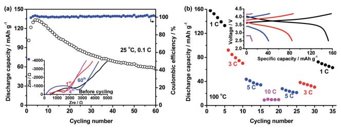
Fig. 7 (a) Cycling performance of the NCM-811/SPE/Li battery at 25 °C and 0.1C. Inset shows the EIS spectra of the battery before cycling, after 1<sup>st</sup> cycle and after 60 cycles. (b) Rate performance of the NCM-811/SPE/Li battery at 100 °C. Inset presents the charge/discharge curves at different rates
