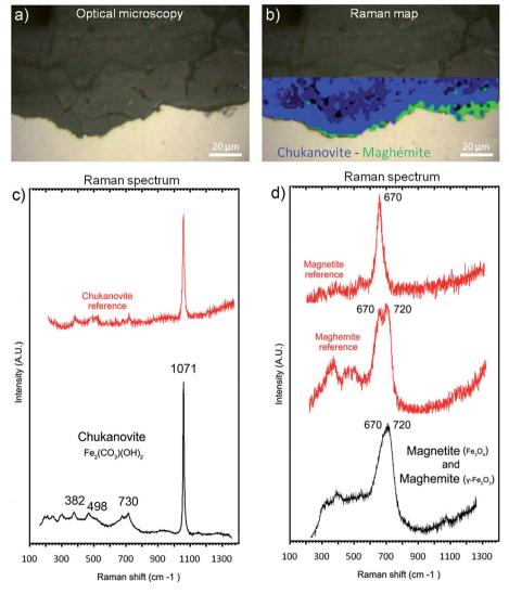
Fig. 10 (a) Optical microscopy photograph and (b) μRaman map of chukanovite (in blue) and magnetite (in green) of the metal/corrosion product interface in a cross-section of the Batx sample. Also shown are representative μRaman spectra of some corrosion products: (c) chukanovite Raman spectra of the internal layer of corrosion products and (d) mixed magnetite-maghemite Raman spectra of the interfacial layer.
