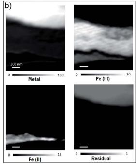
Fig. 14 STXM characterization of the Batx interfacial thin film. (a) Image difference map (290-280 eV) of the thin film obtained from the carbonate spectra collected at the C K-edge. (b) SDV component maps of the Fe(III), Fe(III) and Fe(O) species obtained with the siderite, maghemite and metal reference spectra in part of the thin film (the grey scales indicate the equivalent thickness (nm) on the Fe(O), Fe(III), and Fe(IIII) component maps and the optical density on the residual map).
