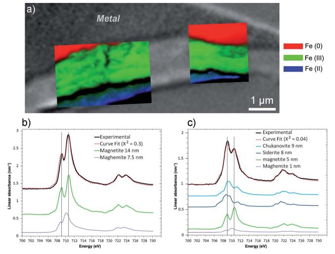
Fig. 15 STXM characterization of the thin film for the Batx sample. (a) Composite color-coded maps of the Fe<sup>(II)</sup> and Fe<sup>(III)</sup> components based on SDV maps of various regions of the thin film superimposed on the image presented in Fig. 14a. Curve fits of the average spectrum obtained on the (b) interfacial and (c) outer layers, along with the reference spectra used (metal, chukanovite, siderite, magnetite and maghemite) and the equivalent thicknesses deduced (in nm).
