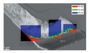
Fig. 5 STXM characterization of the thin film for the Arcorr2008 sample: color-coded  $Fe^{(0)}$ ,  $Fe^{(II)}$  and  $Fe^{(III)}$  component maps (SDV) of various regions superimposed on an image difference map (290–280 eV) of the thin film, based on the carbonate spectra acquired at the C K-edge.
