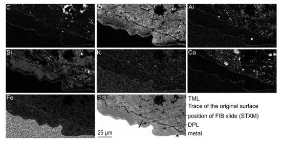
Fig. 1 SEM-BSE image and EDX elemental maps of the Arcorr2008 corrosion interface. The thick segment marks the approximate location of the thin section used in the STXM studies.
