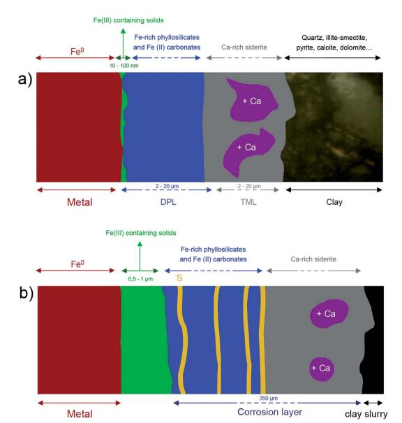
Fig. 16 Diagram of the corrosion patterns at work in the two systems (a) Arcorr2008 and (b) Batx.
