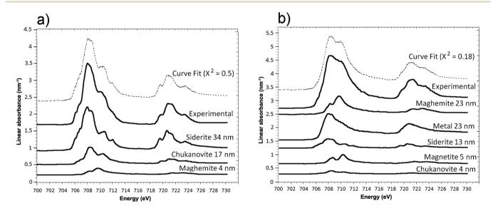
Fig. 6 STXM characterization of the thin film for the Arcorr2008 sample: curve fits of the average spectra obtained on the outer (a) and interfacial (b) layers.
