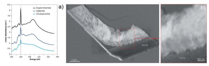
Fig. 3 STXM characterization on the interfacial film between iron and corrosion products for the Arcorr2008 sample. (a) Spectrum extracted from the carbonate zone compared to siderite and chukanovite as references at the C K edge. (b) Image difference map (290–280 eV) of the thin film obtained from the carbonate spectra acquired at the C K edge.
