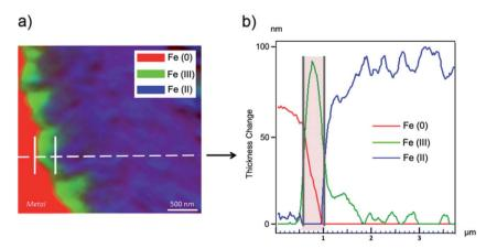
Fig. 7 STXM studies of the thin film for the Arcorr2008 sample: (a) color-coded Fe<sup>(0)</sup>, Fe<sup>(II)</sup> and Fe<sup>(III)</sup> composite map and (b) profile of the line giving the thicknesses of each component, point by point (every 10 nm) around the metal interface.
