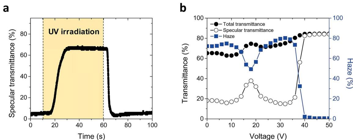
Fig. 5 (a) Changes in specular transmittance of fabricated ChLC cell by UV irradiation at  $30^\circ\text{C}$ . (b) Total transmittance, specular transmittance, and haze of fabricated ChLC cell as functions of the applied voltage.
