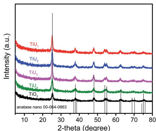
Fig. 1 XRD patterns of TiO<sub>2</sub> and U-doped TiO<sub>2</sub> (TiU<sub>x</sub>,  $x = 1, 2, 3$ , and 4).
