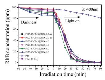
Fig. 10 Adsorption property and photocatalytic activity of various samples towards the degradation of RhB irradiated with visible light  $(400 < \lambda < 680 \text{ nm})$ .
