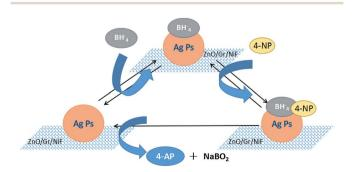
Fig. 6 Schematic showing the 4-NP molecule reduction using the AgNP/ZnO/Gr/NiF hybrid in the presence of NaBH<sub>4</sub> in aqueous medium.
