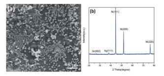
(a) SEM image and (b) XRD pattern of AgNP/ZnO/Gr/NiF hybrid after the catalytic reaction.
