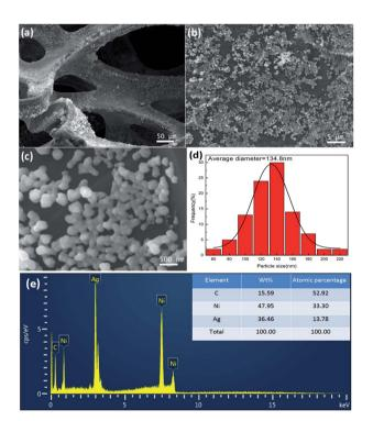
**Fig. 2** (a–c) SEM images of AgNP/ZnO/Gr/NiF hybrids at different magnifications. (d) Particle size distribution of the Ag particles. (e) EDX spectrum of AgNP/ZnO/Gr/NiF.
