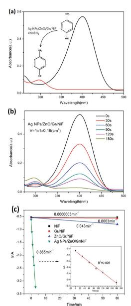
Fig. 5 (a) UV-vis absorption spectra of 4-NP and 4-AP. (b) Successive UV-vis absorption spectra of the reduction of 4-NP using NaBH<sub>4</sub> in the presence of the AgNP/ZnO/Gr/NiF hybrid. (c) The logarithm of the absorbance at 400 nm versus reduction time and the enlarged drawing (inset) of AgNP/ZnO/Gr/NiF with the error bars.
