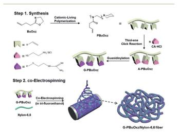
Scheme 1 Synthesis of G-PBuOxz and the co-electrospinning of G-PBuOxz/Nylon-6,6 fibers.
