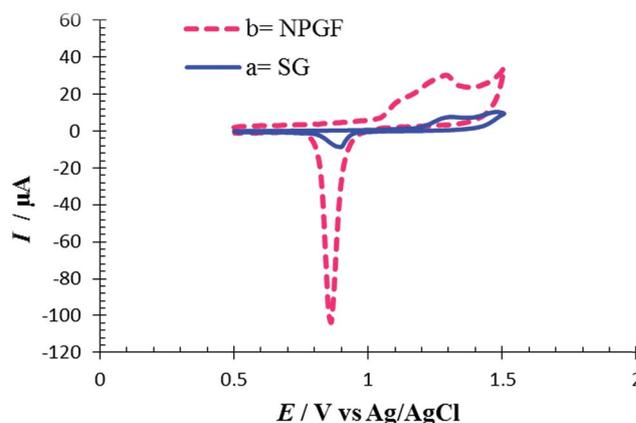
Fig. 1 Cyclic voltammograms for (a) SG electrode and (b) a NPGF electrode in 0.5 mol L<sup>-1</sup> H<sub>2</sub>SO<sub>4</sub> solution. Scan rate 10 mV s<sup>-1</sup>.
