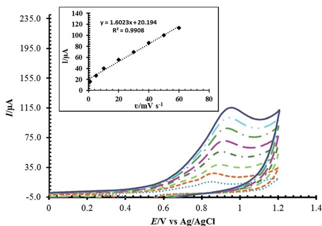
Fig. 9 Cyclic voltammograms of RuPtNPGF electrode in the presence of  $100 \mu\text{mol L}^{-1}$  Met in  $0.1 \text{ mol L}^{-1}$  phosphate buffer ( $\text{pH} = 7$ ) solution at various scan rates  $5\text{--}60 \text{ mV s}^{-1}$ .
