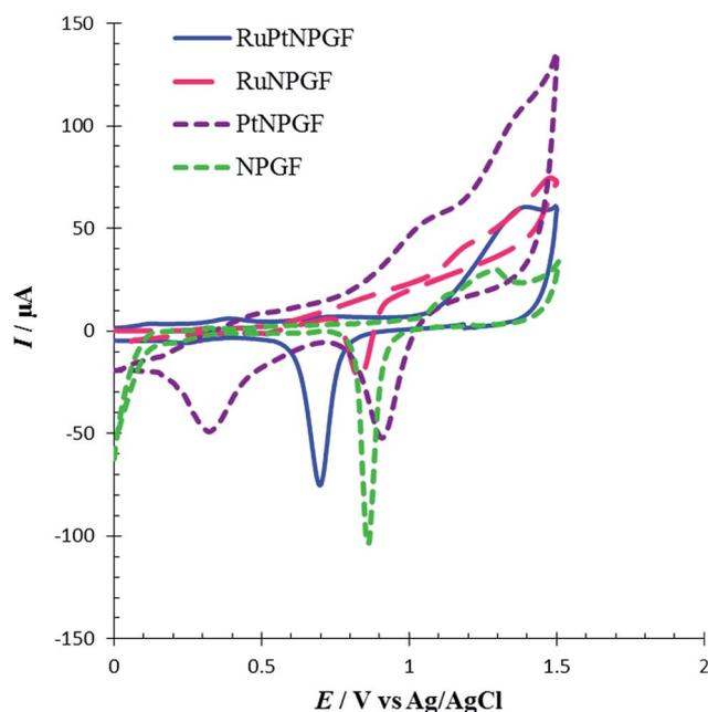
Fig. 5 Cyclic voltammograms for NPGF, PtNPGF, RuNPGF and RuPtNPGF electrodes in 0.5 mol L<sup>-1</sup> H<sub>2</sub>SO<sub>4</sub> solution. Scan rate 10 mV s<sup>-1</sup>.
