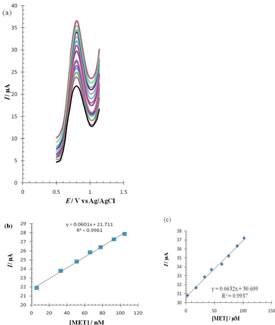
Fig. 13 (a) Differential pulse voltammograms of Met under optimum conditions; (b) shows plot of 6, 33, 51, 66, 78, 93, 105  $\text{nmol L}^{-1}$  of Met and (c) shows plot of 3, 18, 33, 45, 63, 75, 90, 102  $\mu\text{mol L}^{-1}$  of Met in phosphate buffer solution (pH = 7, 0.1  $\text{mol L}^{-1}$ ).
