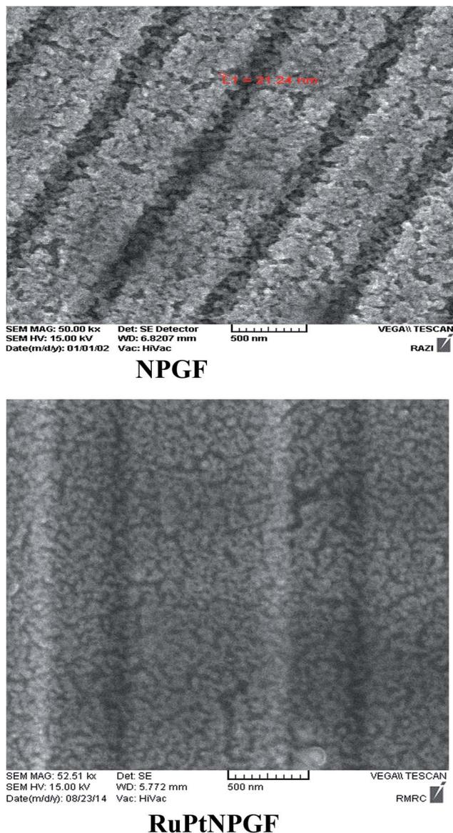
Fig. 3 SEM image of NPGF and RuPtNPGF electrodes.
