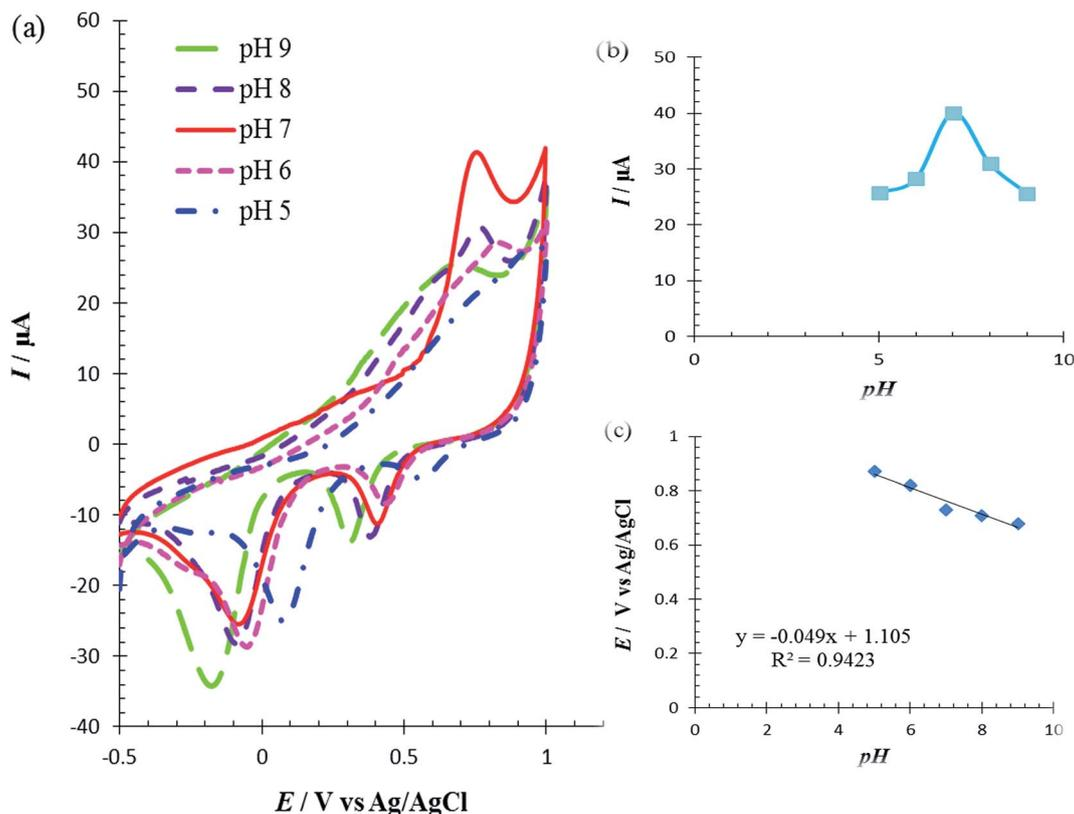
Fig. 8 (a) Cyclic voltammograms (b) the effect of pH on anodic peak current (c) the influence of pH on anodic peak potential for oxidation of  $100 \mu\text{mol L}^{-1}$  Met at the surface of the RuPtNPGF electrode at various pH (5–9) in  $0.1 \text{ mol L}^{-1}$  phosphate buffer solution. Scan rate  $10 \text{ mV s}^{-1}$ .
