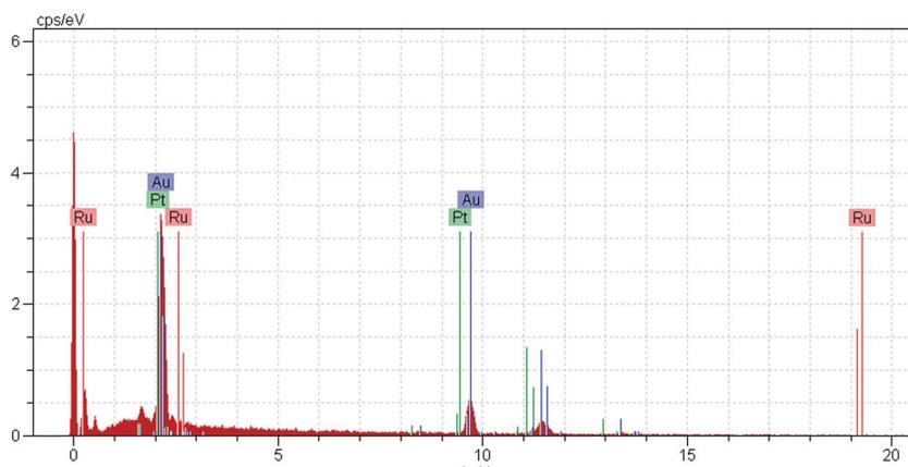
Fig. 4 EDX pattern of RuPtNPGF electrode.
