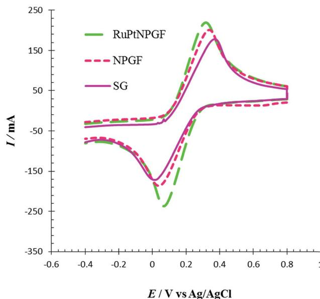
Fig. 6 Cyclic voltammograms for SG, NPGF and RuPtNPGF electrodes in 5 mM K<sub>3</sub>[Fe(CN)<sub>6</sub>] + 5 mmol L<sup>-1</sup> K<sub>4</sub>[Fe(CN)<sub>6</sub>] contained in 0.1 mol L<sup>-1</sup> NaNO<sub>3</sub> solution. Scan rate 10 mV s<sup>-1</sup>.
