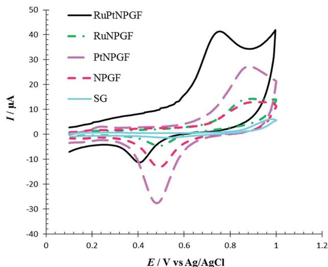
Fig. 10 Cyclic voltammograms for oxidation of  $100 \mu\text{mol L}^{-1}$  Met at the surface of SG, NPGF, PtNPGF, RuNPGF and RuPtNPGF electrodes in  $0.1 \text{ mol L}^{-1}$  phosphate buffer ( $\text{pH} = 7$ ) solution. Scan rate  $10 \text{ mV s}^{-1}$ .
