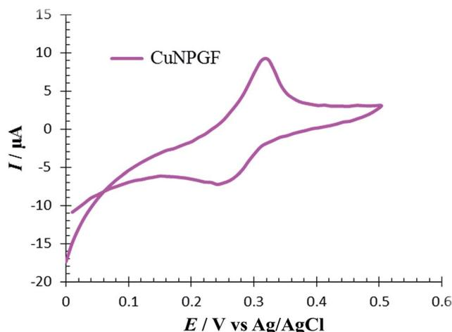
Fig. 2 Cyclic voltammogram for CuNPGF electrode in 0.5 mol L<sup>-1</sup> H<sub>2</sub>SO<sub>4</sub> solution. Scan rate 10 mV s<sup>-1</sup>.
