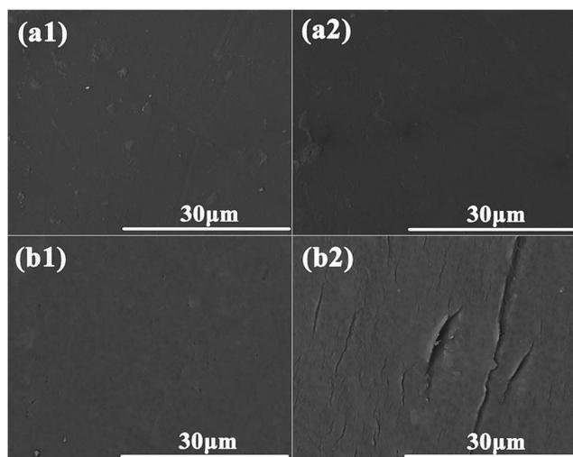
Fig. 13 The outer surface morphologies of the BR PMIA and commercial PVDF membranes following the thermal rejection process for: (a) the BR PMIA membranes, (b) the commercial PVDF membranes, where: (1) the operation temperature was 25 °C, (2) the operation temperature was 90 °C.
