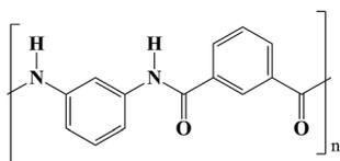
Fig. 1 Chemical structure of PMIA.
