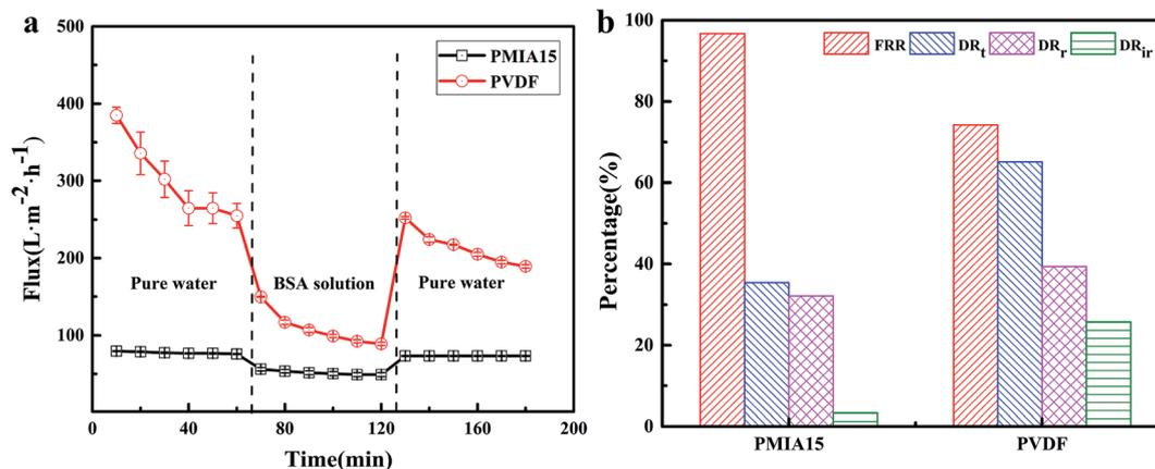
Fig. 11 Time-dependent permeate flux of PMIA15 membranes and commercial PVDF membranes (a), and the summary of the corresponding FRR, DR<sub>t</sub>, DR<sub>r</sub>, DR<sub>ir</sub> values (b) during BSA solution filtration.
