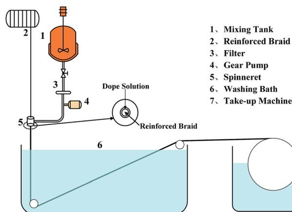
Fig. 3 Schematic diagram of the dry-wet spinning apparatus.
