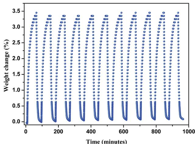
Fig. 7 CO<sub>2</sub> adsorption/desorption cycles obtained for the compound **1** from 25 to 80 °C.
