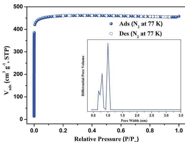
Fig. 5 N<sub>2</sub> adsorption and desorption isotherms at 77 K. Inset: pore size distribution of compound **1**.
