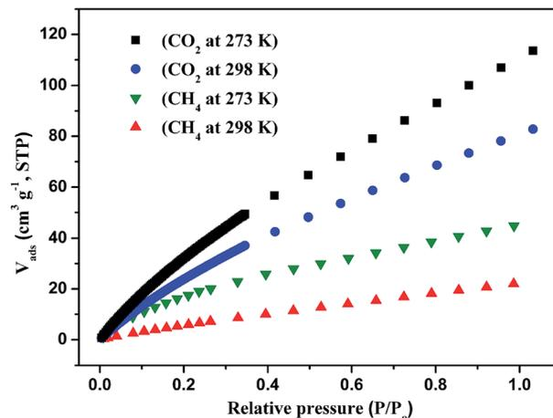
Fig. 6 CO<sub>2</sub> and CH<sub>4</sub> adsorption isotherm of compound **1** at 273 K and 298 K.
