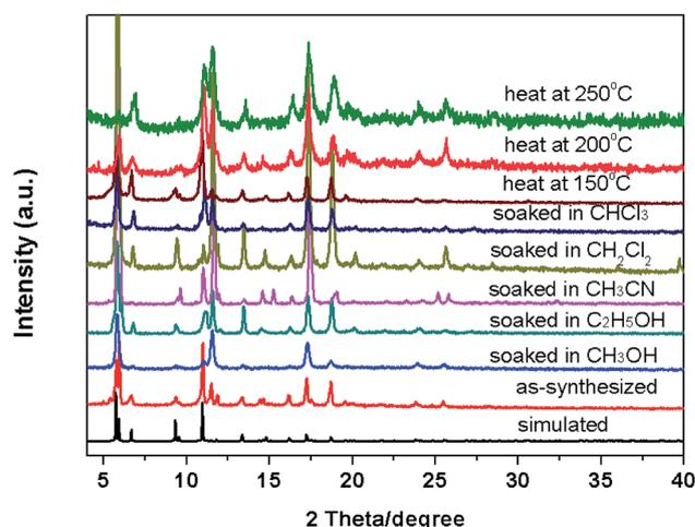
Fig. 4 The PXRD patterns for compound **1** soaked in different solvents and heat in variable temperature.
