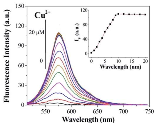
Fig. 3 The fluorescence intensity change profile of sensor 1 ( $1 \mu\text{M}$ ) to different metal ions (1 mM) in 0.1 M Tris–HCl solution (ethanol–water = 1 : 10, v/v, pH 7.14,  $\lambda_{\text{ex}} = 500 \text{ nm}$ ). Inset: corresponding fluorescent spectra of 1 in the presence of different concentrations  $\text{Cu}^{2+}$  ions.
