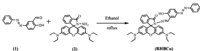
Scheme 1 Synthesis and structure of sensor 1.
