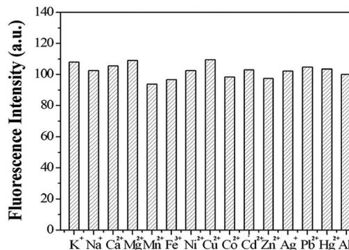
Fig. 9 The fluorescence intensity of sensor 1 ( $\mu\text{M}$ ) with 1.5 equiv. of  $\text{Cu}^{2+}$ , followed by 10 equiv. of  $\text{M}^{n+}$ . (Tris-HCl, pH 7.14, ethanol-water = 1 : 10, v/v,  $\lambda_{\text{ex}}$  = 500 nm).
