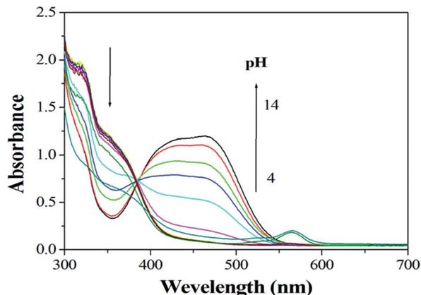
Fig. 1 Absorption of sensor 1 with different pH.
