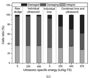
Fig. 4 Damage to EPS (a), cell walls (b) and cell membranes (c) of combined 0.04 g  $\rm g^{-1}$ -TS lime with different ultrasound specific energy input.
