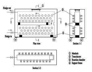
Fig. 1 Diagram of full-scale ultrasonic bath reactor.
