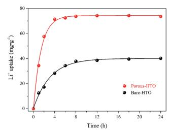
Fig. 5 Li<sup>+</sup> uptake kinetics of both bare-HTO and porous-HTO in the simulation Bayer liquor.
