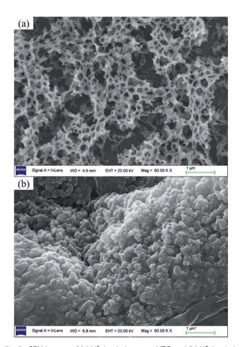
Fig. 8 SEM images of (a) Li $^+$ -loaded porous-HTO and (b) Li $^+$ -loaded bare-HTO after 5 cycle operation.
