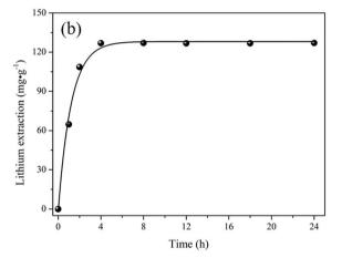
Fig. 1 (a) Lithium extraction and dissolution of titanium upon treatment of porous-LTO with different HCl solutions; (b) the lithium extraction rate from porous-LTO with 0.2 mol  $\rm L^{-1}$  HCl solution.
