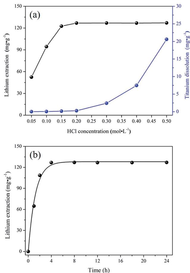
Fig. 1 (a) Lithium extraction and dissolution of titanium upon treatment of porous-LTO with different HCl solutions; (b) the lithium extraction rate from porous-LTO with 0.2 mol L<sup>-1</sup> HCl solution.
