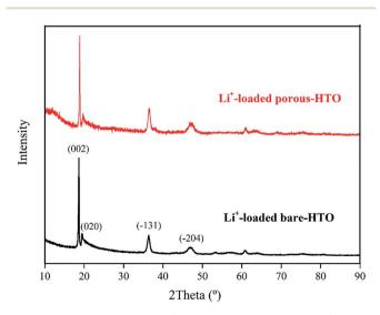
Fig. 7 XRD patterns of both Li<sup>+</sup>-loaded porous-HTO and Li<sup>+</sup>-loaded bare-HTO after 5 cycle operation.
