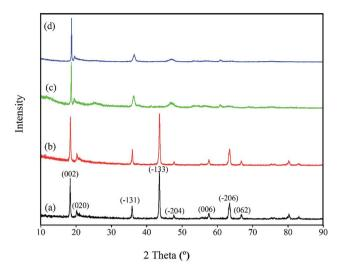
Fig. 2 XRD patterns of (a) the bare-LTO, (b) the porous-LTO, (c) the bare-HTO, and (d) the porous-HTO.
