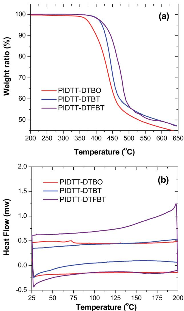
Fig. 1 TGA and DSC plot of polymers with a heating rate of 10 °C min<sup>-1</sup> under a nitrogen atmosphere.
