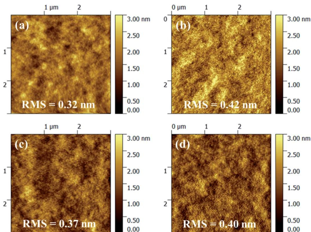
Fig. 6 Tapping mode AFM topography images ( $3 \times 3 \mu\text{m}^2$ ) of polymer/PC<sub>71</sub>BM blend films, (a) **PIDTT-DTBO**/PC<sub>71</sub>BM before annealing. (b) **PIDTT-DTBO**/PC<sub>71</sub>BM after annealing at 100 °C for 10 min (c) **PIDTT-DTBT**/PC<sub>71</sub>BM before annealing. (d) **PIDTT-DTBT**/PC<sub>71</sub>BM after annealing at 100 °C for 10 min.
