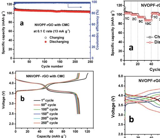
Fig. 6 (a) Cycling performance and (b) charge—discharge cycles of the NVOPF—rGO composite with a CMC-Na binder for 250 cycles.
