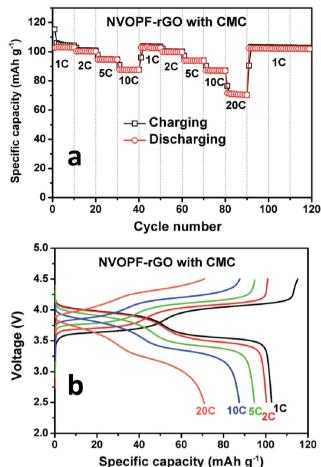
Fig. 7 (a) Rate capability and (b) charge-discharge cycles of the NVOPF-rGO composite with CMC at different C-rates.
