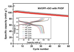
Fig. 4 Cyclability of the NVOPF-rGO cathode with a PVDF binder in a Na half-cell for 60 cycles. The charge/discharge curves are shown in the inset figure.
