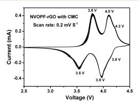
Fig. 5 The CV plot for the NVOPF-rGO composite with a CMC-Na binder for 20 cycles at a scan rate of 0.2 mV  $\rm S^{-1}$ .
