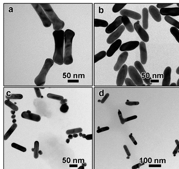
Fig. 4 TEM images of Au nanostructures obtained by varying the reaction parameters. (a and b) The concentration of PSS was: (a)  $0 \text{ mg mL}^{-1}$ , (b)  $3 \text{ mg mL}^{-1}$ , the concentration of NaOH was: (c)  $0 \text{ mM}$ ; (d)  $1.0 \text{ mM}$ .
