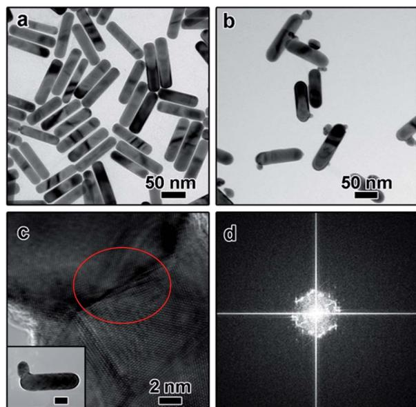
Fig. 1 TEM images of (a) Au nanorods; (b) AuNR–AuNP dimer after treated with PSS (the final concentration of PSS was  $10 \text{ mg mL}^{-1}$ ); (c) HR-TEM image of the enlarged interface region. The inset shows the corresponding low-magnification TEM. (d) FFT diffractogram corresponding to the area marked by the red circle in (c). The scale bar in the inset of (c) is 20 nm.
