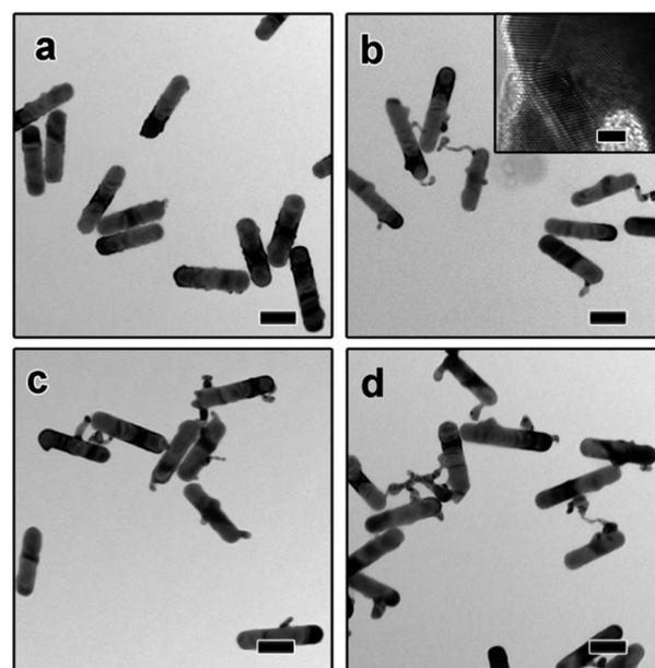
Fig. 2 TEM images of AuNR–AuNP dimers obtained after reacted for different time: (a) 15 min (b) 30 min, (c) 45 min (d) 60 min. The inset in (b) is the corresponding HR-TEM image. The scale bars in (a–d) and the inset of (b) are 50 nm and 2 nm, respectively.
