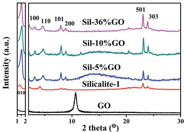
**Fig. 1** XRD of GO dried at 50 °C, silicalite-1, Sil-5% GO, Sil-10% GO and Sil-36% GO composites synthesized at 150 °C for 8 d. The scans were done in in-plane mode with  $2\theta$  varying from 1° to 30° with a step size of 0.02° and dwell time of 0.4 s at room temperature. The gap at 2°  $2\theta$  was as-broken for clear observation of the special peaks from 2–30°.
