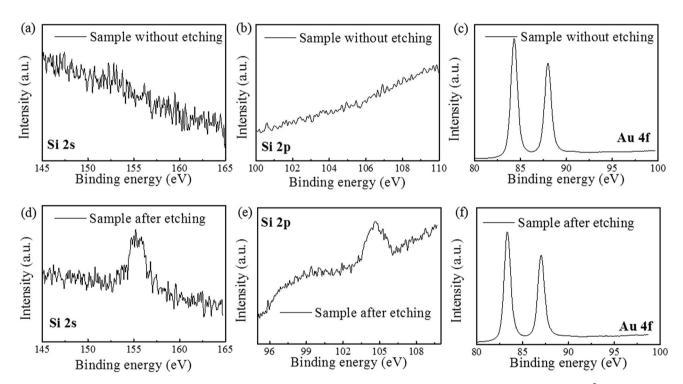
Fig. 5 XPS result on the Au film surface (a–c) before etching and (d–f) after etching. (a), (b), (d) and (e) show the change of  $SiF_6^{2-}$  and  $SiO_2$ ; (c) and (f) show the shift of the peak of Au 4f.
