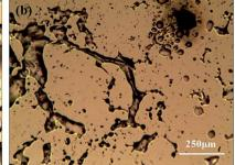
Fig. 6 Optical image of the assemble of  $H_2$  under the Au film and the damage of the Au film caused by the release of  $H_2$  (a) optical image in the center area of the  $H_2$  bubble; (b) optical image in marginal area.
