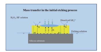
Fig. 7 Schematic image of mass transfer during the initial etching process. The reaction occurs at the interface of Au film and solution: Si atoms diffuse through the Au film and produce to  $H_2SiF_6$  on the surface of Au film;  $H^+$  in some way diffuses through the Au film and produces the  $H^2$  at the Au/Si interface.
