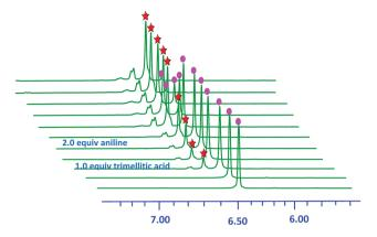
Fig. 1 Partial 400 MHz  $^1$ H NMR spectra (D<sub>2</sub>O) of a mixture of Cp<sub>2</sub>ZrCl<sub>2</sub> (1.0 equiv.) and trimellitic acid (1.0 equiv.) with PhNH<sub>2</sub> (2.0 equiv). 6.49 ppm  $I \bullet [Cp_2ZrCl_2]$ ; 6.57 ppm  $I \bullet Cp_2Zr(OOC)_2$ PhCOOH.
