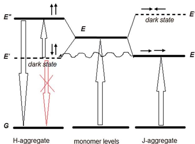
Fig. 5 Proposed energy scheme of the upconversion.
