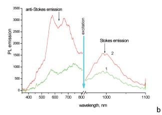
Fig. 2 PL emission spectra of (a) aqueous solutions of (1) neat dye 1859SL ( $10^{-5}$  M), (2) dye: ErCl<sub>3</sub> mixture ( $10^{-5}$ :  $10^{-1}$  molar ratio), (3) ErCl<sub>3</sub> ( $10^{-1}$  M) and (b) films of (1) neat dye 1859SL, (2) dye–ErCl<sub>3</sub> composite (1:1 molar ratio). Excitation band is indicated on the graphs by a blue arrow, and the insert in (a) shows the actual transmission spectrum of the excitation light from the halogen lamp through corresponding filters.
