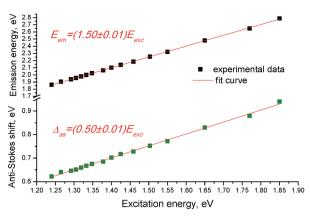
Fig. 4 Dependence of the anti-Stokes shift  $\Delta_{\rm as}$  (lower data) and the anti-Stokes emission energy  $E_{\rm em}$  (upper data) on the excitation energy  $E_{\rm exc}$  in the films of 1859SL. The solid lines are the linear fit of the experimental results.
