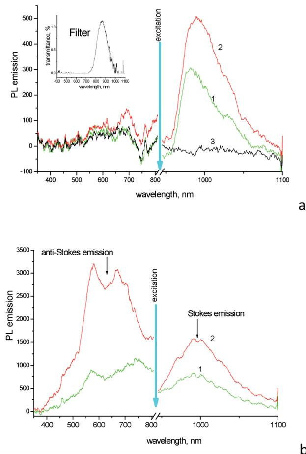
Fig. 2 PL emission spectra of (a) aqueous solutions of (1) neat dye 1859SL ( $10^{-5}$  M), (2) dye :  $\text{ErCl}_3$  mixture ( $10^{-5}$  :  $10^{-1}$  molar ratio), (3)  $\text{ErCl}_3$  ( $10^{-1}$  M) and (b) films of (1) neat dye 1859SL, (2) dye- $\text{ErCl}_3$  composite (1 : 1 molar ratio). Excitation band is indicated on the graphs by a blue arrow, and the insert in (a) shows the actual transmission spectrum of the excitation light from the halogen lamp through corresponding filters.
