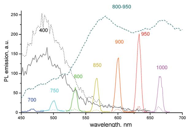
Fig. 3 PL emission spectra of the neat dye 1859SL (dotted curves) and the dye- $\text{CaCl}_2$  composite (1 : 5 molar ratio, solid curves) films. The excitation wavelengths are indicated near each curve. The results are compared to the upconversion emission of the films upon the broadband excitation at 800–950 nm (dashed curve, see also Fig. 2b).
