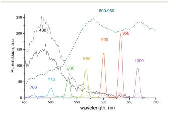
Fig. 3 PL emission spectra of the neat dye 1859SL (dotted curves) and the dye-CaCl<sub>2</sub> composite (1:5 molar ratio, solid curves) films. The excitation wavelengths are indicated near each curve. The results are compared to the upconversion emission of the films upon the broadband excitation at 800–950 nm (dashed curve, see also Fig. 2b).
