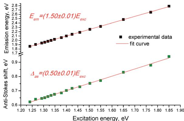
Fig. 4 Dependence of the anti-Stokes shift  $\Delta_{as}$  (lower data) and the anti-Stokes emission energy  $E_{em}$  (upper data) on the excitation energy  $E_{exc}$  in the films of 1859SL. The solid lines are the linear fit of the experimental results.
